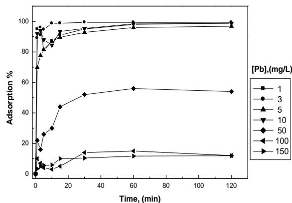
Fig. 2: Adsorption % of Pb<sup>2+</sup> concentration (mg l<sup>-1</sup>) on SWM at different shaking times.
