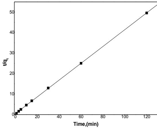
Fig. 4: Plot of  $(t/q_t)$  vs. stirring time ( $t$ ) for the adsorption of  $Pb^{2+}$  by 0.1 g SWM at pH 6.
