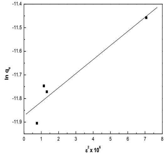
Fig. 7: D-R isotherm for  $Pb^{2+}$  adsorption onto SWM
