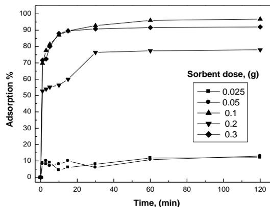
Fig. 3: Effect of SWM dose on adsorption % of Pb<sup>2+</sup> at
