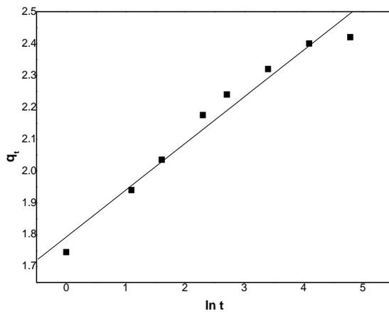
Fig. 5: Plot of  $q_t$  vs.  $\ln t$  for the adsorption of  $Pb^{2+}$  by 0.1 g SWM at pH 6.
