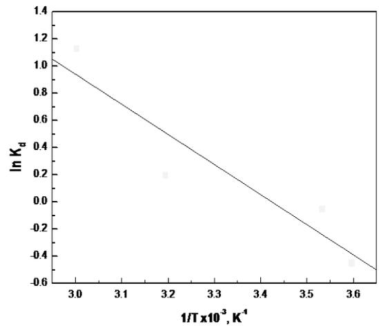
Fig. 8: Thermodynamic distribution coefficient ( $K_d$ ) calculated for the adsorption of  $Pb^{2+}$  on SWM as a function of temperature.
