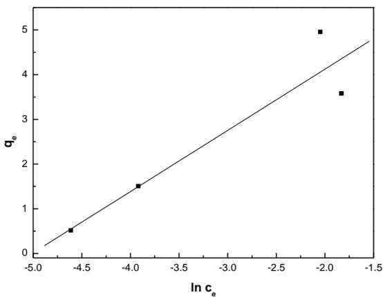
Fig. 6: Plot of  $q_e$  vs.  $\ln c_e$  for the adsorption of  $Pb^{2+}$  by 0.1 g SWM at pH 6.
