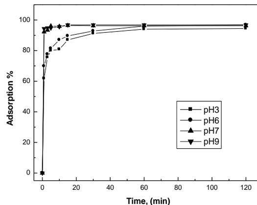
Fig. 1: Adsorption % of 5 mg l<sup>-1</sup> Pb<sup>2+</sup> by 0.1 g SWM vs shaking time at different pH's.
