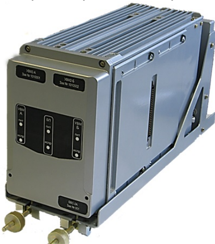
Figure 5. Example of a military electronic safe design with a locking mechanism on the front for easy assembly and disassembly [© https://tridentinfosol.com ]
