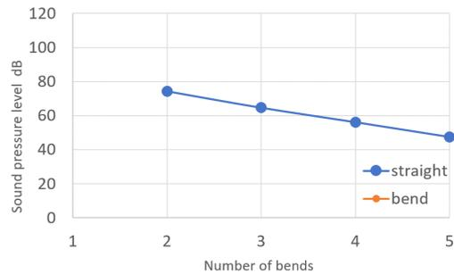
Figure 16 Peak sound pressure level of 1<sup>st</sup> mode in case of 0.04m square and with absorbent
