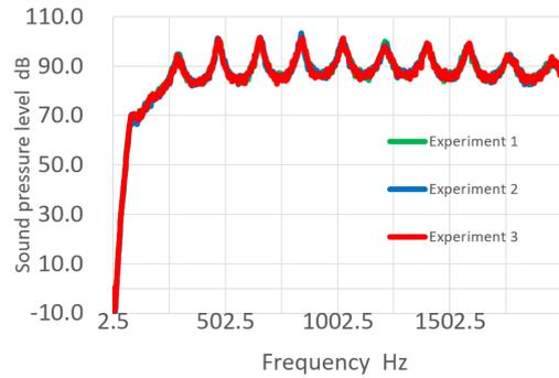
Figure 4 FFT result for three straight ducts with 0.05m square
