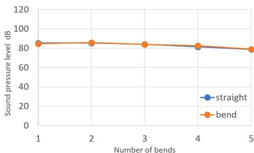
Figure 23 Peak sound pressure level of 4<sup>th</sup> mode
