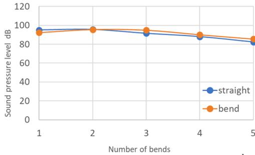
Figure 14 Peak sound pressure level of 3<sup>rd</sup> mode
