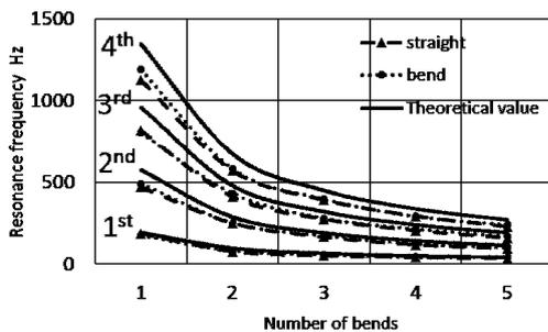
Figure 8 Resonant frequencies of duct with 0.065m square in case of with absorbent.
