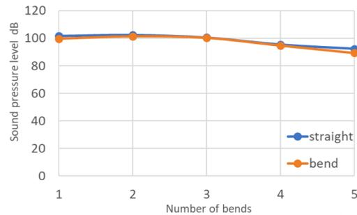
Figure 10 Peak sound pressure level of 3<sup>rd</sup> mode
