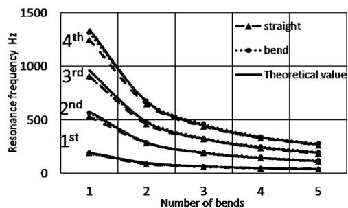
Figure 6 Resonant frequencies of ducts with 0.075 square in case of without absorbent.
