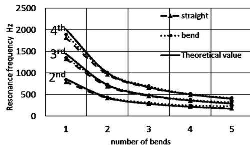
Figure 5 Resonant frequencies of ducts with 0.05m square in case of without absorbent.
