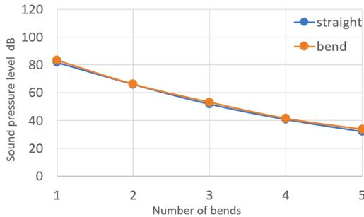
Figure 20 Peak sound pressure level of 1<sup>st</sup> mode
