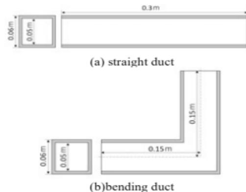
Figure 2 Bending and straight ducts with 0.05m square
