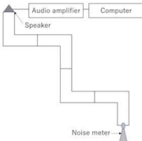
Figure 3 Connected four bending ducts
