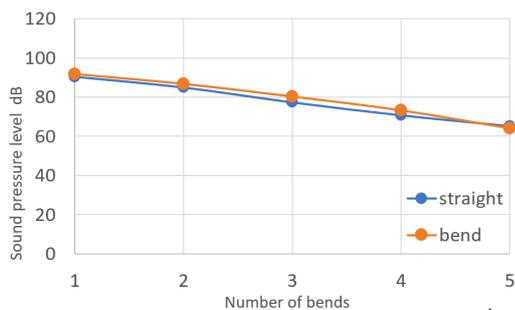
Figure 21 Peak sound pressure level of 2<sup>nd</sup> mode
