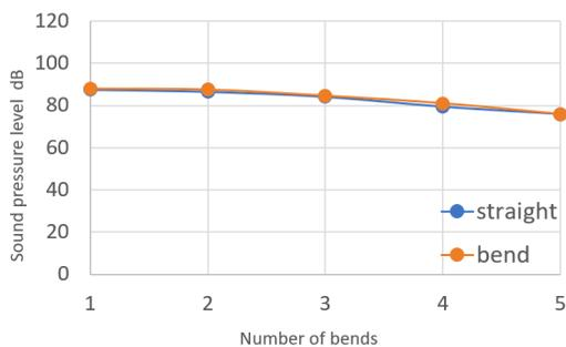
Figure 22 Peak sound pressure level of 3<sup>rd</sup> mode
