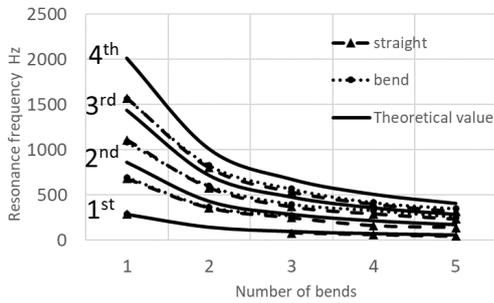
Figure 7 Resonant frequencies of duct with 0.04 square in case of with absorbent.
