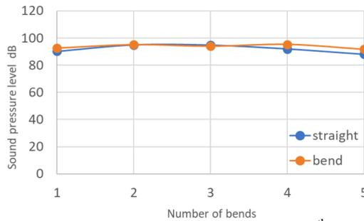
Figure 15 Peak sound pressure level of 4<sup>th</sup> mode in case of 0.075 square and without absorbent
