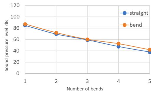
Figure 12 Peak sound pressure level of 1<sup>st</sup> mode
