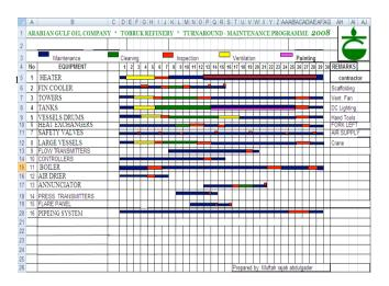
Fig "1": Illustration of The Scheduled Maintenance for The Nine Major Equipment in Tobruk Petroleum Refinery
