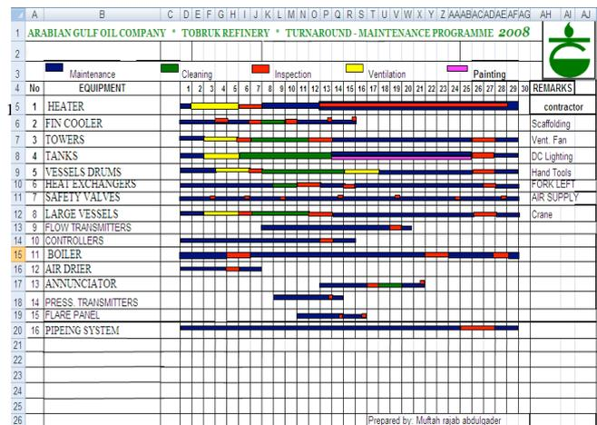
Fig "1": Illustration of The Scheduled Maintenance for The Nine Major Equipment in Tobruk Petroleum Refinery
