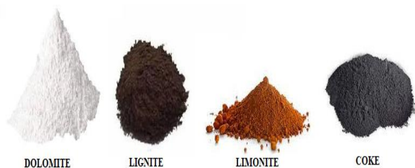
Fig. 1 Image of all sorbent used for defluorination.
