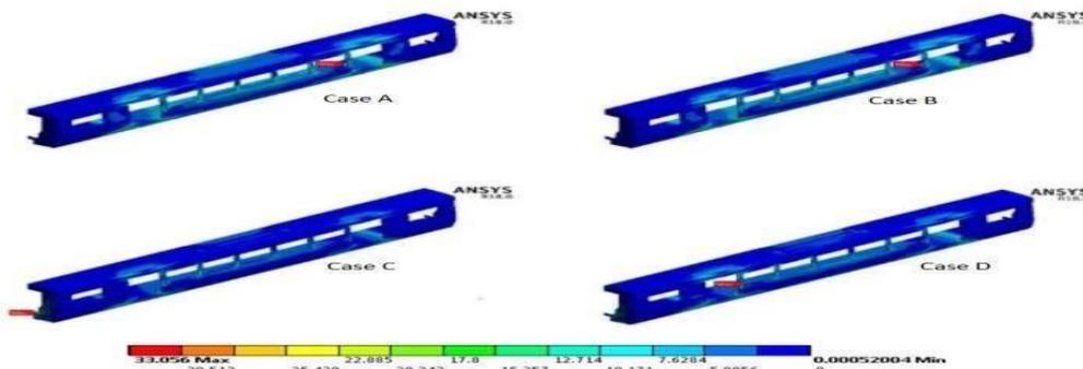
Fig 5: Distribution of von misses under various loading cases for AL6061[5]
