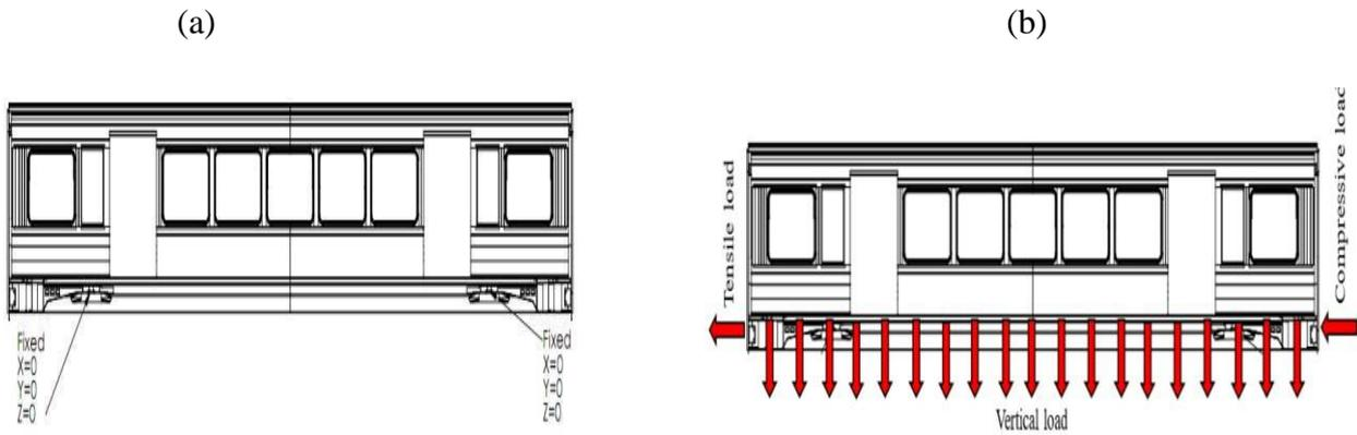
Fig 4: Figures 4a and 4b: Show boundary conditions and location of forces respectively [5]
