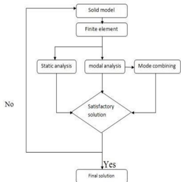
Fig 1: Showing steps for carrying out static structure analysis [2]
