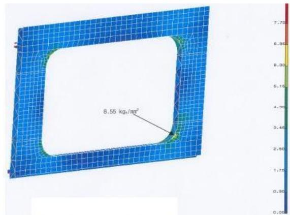
Fig 9a and 9b: Showing maximum stress distribution at the window [6][7]
