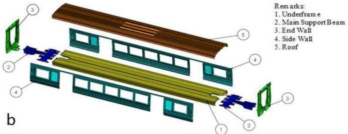
Fig 3: Showing parts of a carbody structure [5]
