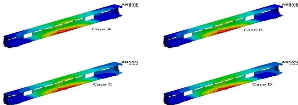
Fig 6: Distribution of von misses stress under various loading cases for Al 6005 [5]
