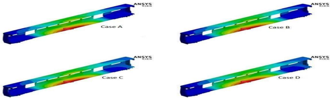
Fig 7: Total deformation results under various load cases for AL6061 [5]
