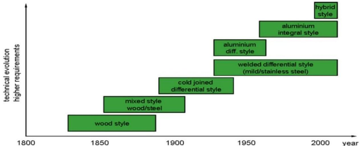
Fig 2: The show the chronology development of rail vehicle body material from the begging of the railcar to the recent history [4]
