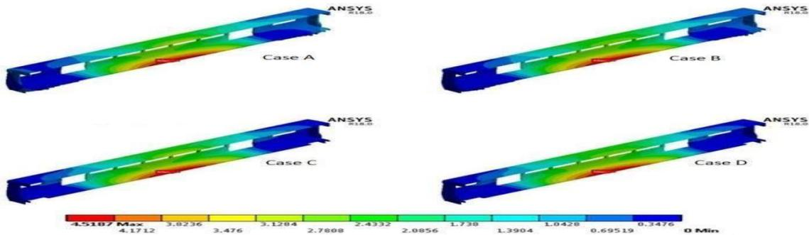
Fig 8: Total deformation results under various load cases for AL6005 [5]
