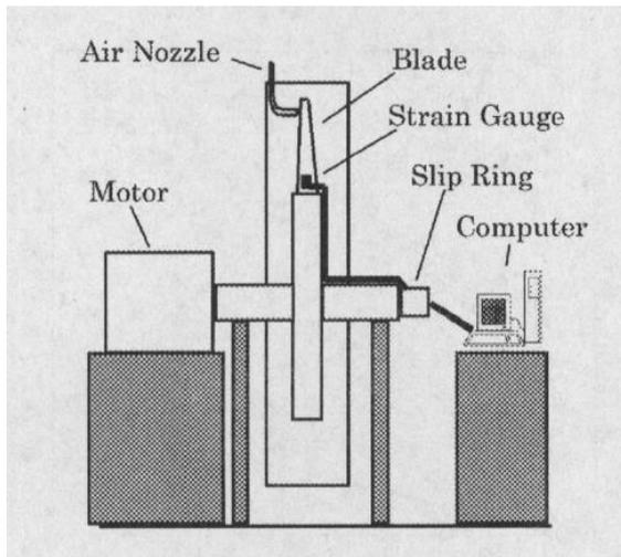
Fig.2 Schematic of test rig
