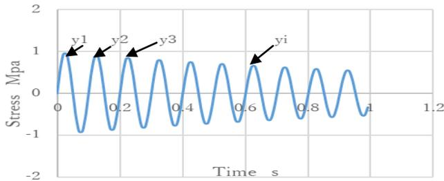
Above figure shows the free damped vibration. The peak values are denoted by  $y_1, y_2, y_3, \dots, y_i, \dots$ , respectively. The logarithmic decrement between adjacent peaks can be given as follows.
