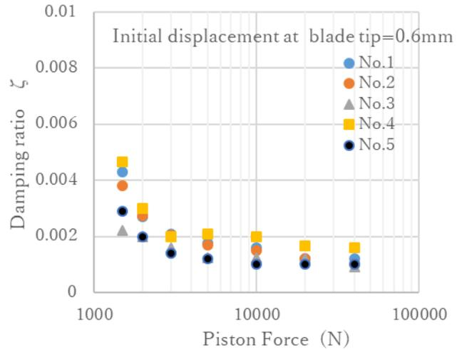
Fig.8 Result of logarithmic damping of test blades
