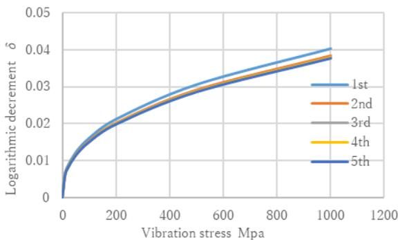
Fig.10 Logarithmic decrement based on specific damping theory
