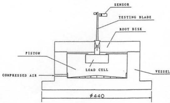
Fig.5 Test rig for obtaining logarithmic damping
