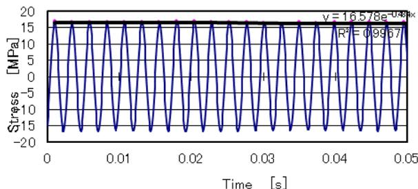
Fig.7 Free damped vibration of test blade enlarged time axis
