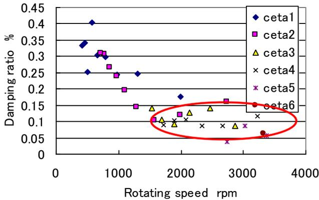
Fig.4 Logarithmic decrement due to rotating test
