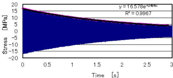
Fig.6 Free damped vibration of test blade
