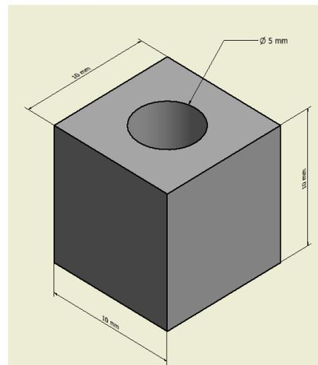
Fig. 1: 3D Print specimen dimensions
