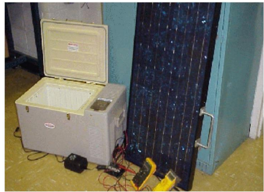
FIG 3 REFRIGERATOR WITH R 134 REFRIGERANT
