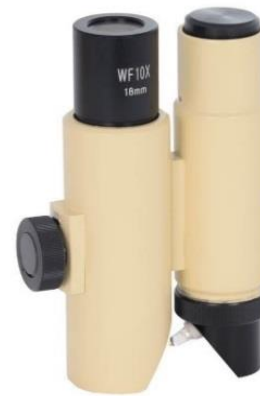
Figure 7. Crack Width Microscope
