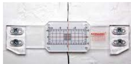
Figure 4: Details and Installation of Plastic Tell-Tale
