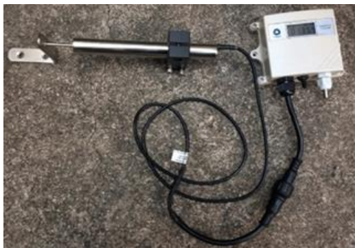
Figure 6: Installation of Linear variable displacement transformer instrument
