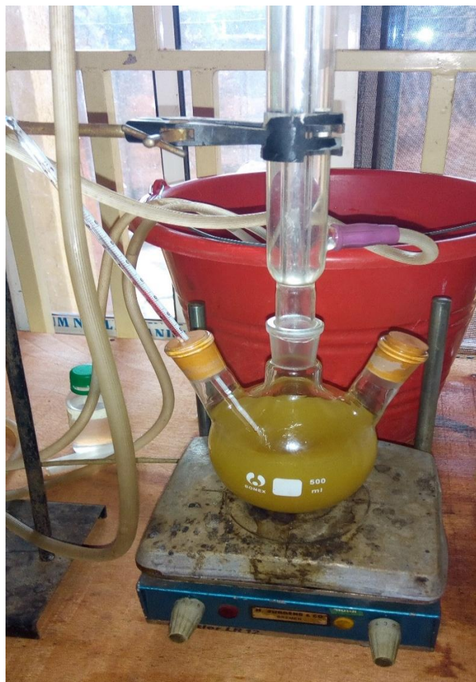
Plate 2: Biodiesel production by transesterification
