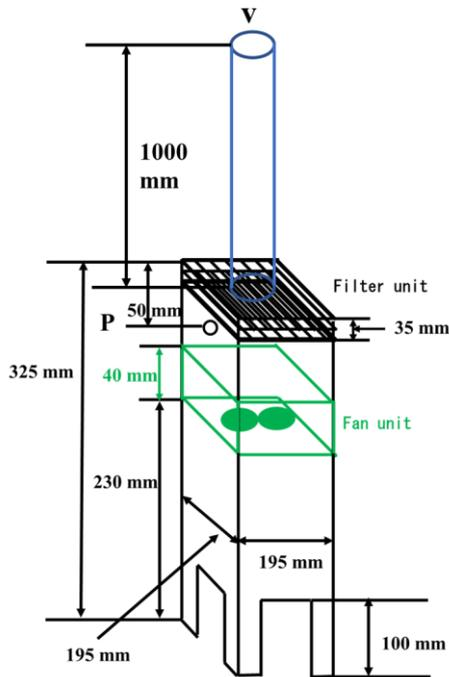
Figure 5. Cylindrical experiment schematic diagram
