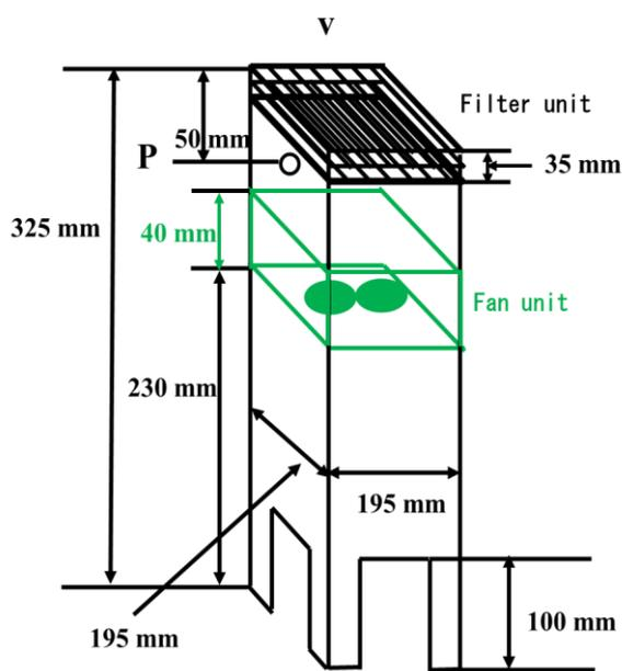
Figure 2. Schematic diagram of experimental equipment.
