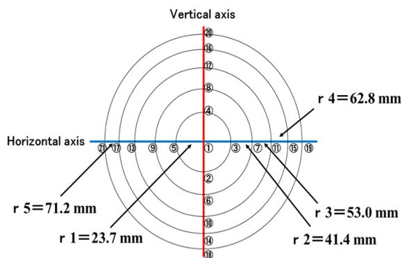
Figure 3. Exit side flow velocity measurement point
