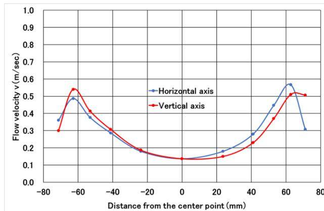
Figure 4. Flow velocity distribution on the outlet side of the deodorizing device
