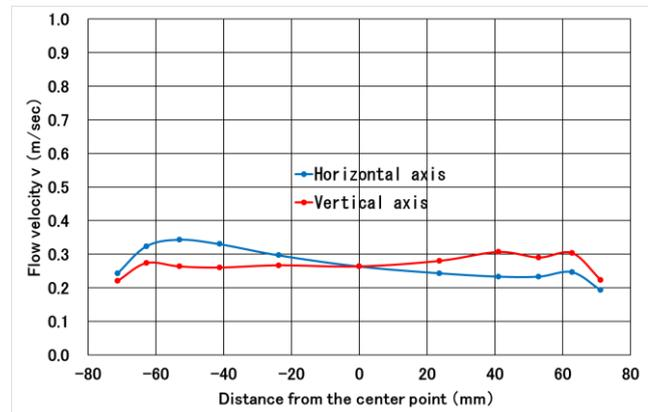
Figure 7. Cylindrical experiment deodorizing device outlet flow velocity distribution
