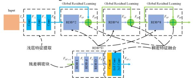
Fig. 7 The process of feature extraction module RDB\*D
