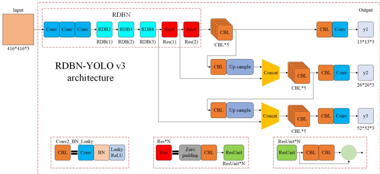
Fig. 5 RDBN-YOLOv3 network structure diagram
