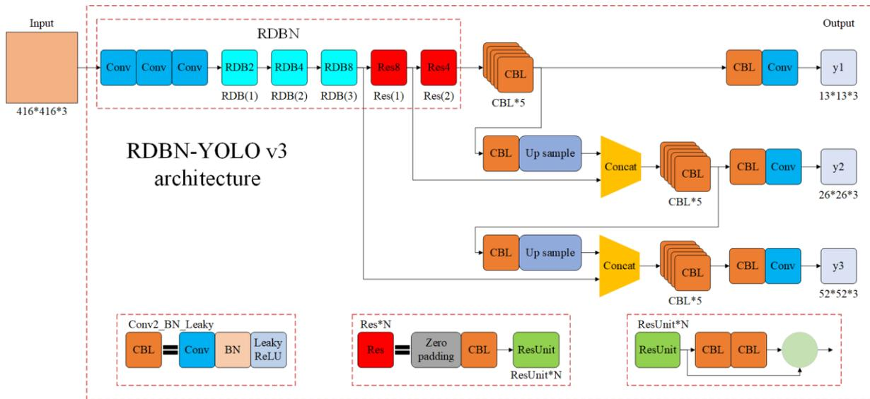
Fig. 5 RDBN-YOLOv3 network structure diagram
