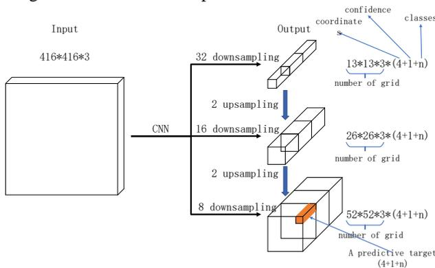
Fig. 2 YOLOv3 Input-Output (regardless of network structure)
