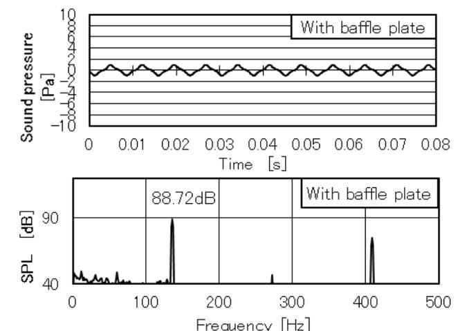
Fig.11 Sound pressure in the case of with the baffle plate.
