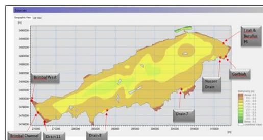
Figure 4: Existing drain sources
