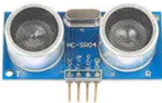
Fig 2: Ultrasonic sensor HC-SR04
