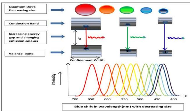
Figure 4: Optical Spectra of Quantum Dots with Decreasing Size (Ikeri and Onyia, 2019).
