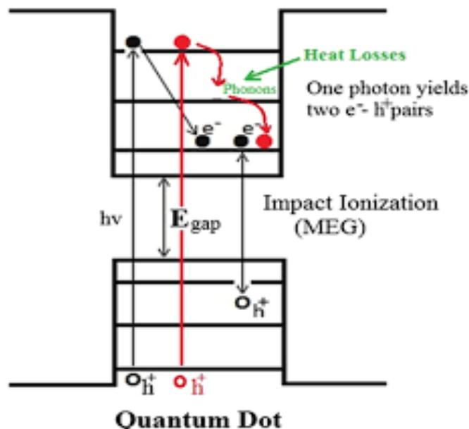
Figure 14 : Multi Exciton Generation Mechanism
