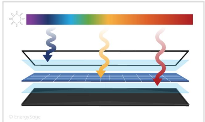
Figure 11: Multi Junction Solar Cell
