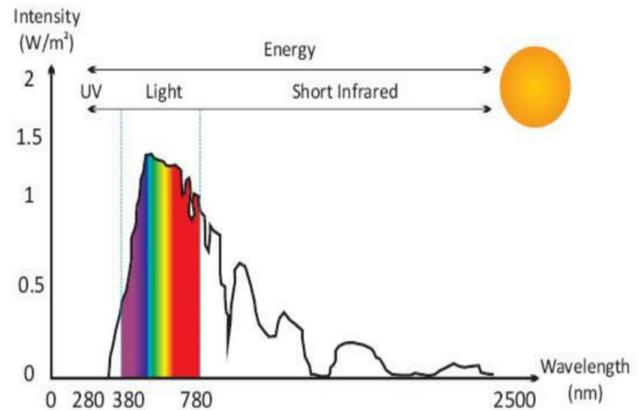
Figure 1: The Solar Energy Distribution Spectrum (Ikeri and Onyia, 2019).
