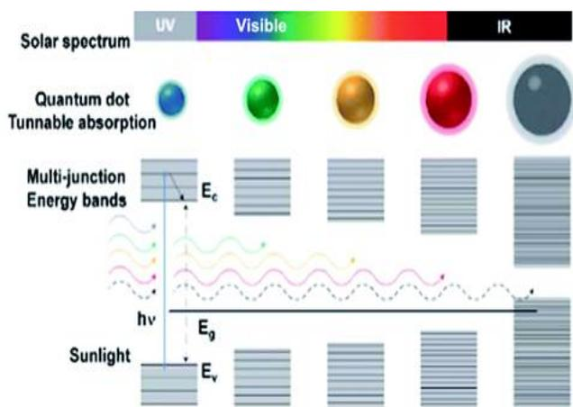
Figure 10: Quantum Dot Multi Junction Energy Band
