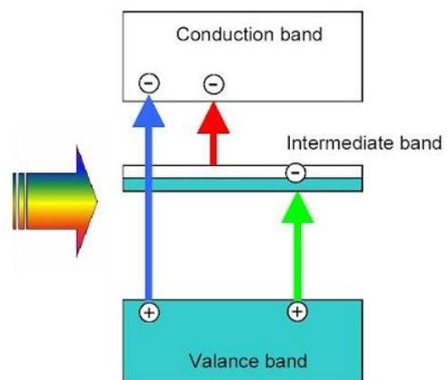
Figure 7: Intermediate Band Solar Cell (Luque and Martin, 2010)
