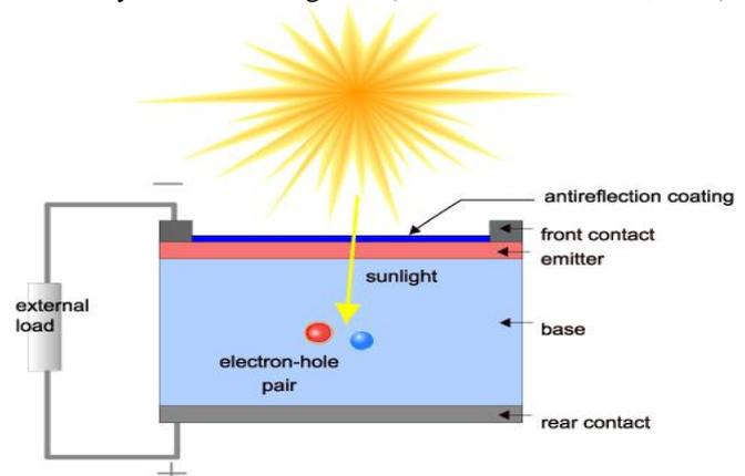
Figure 2: Diagram Showing the Basic Operation of Solar Cell (Jara, 2014)
