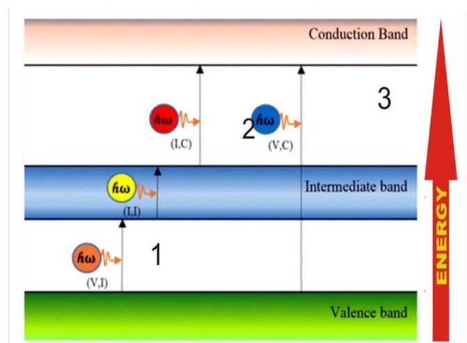
Figure 22: One Intermediate Band Solar Cell Mechanism with the possible Electronic Transitions
