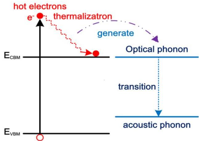
Figure 3: Thermalization of Hot electrons
