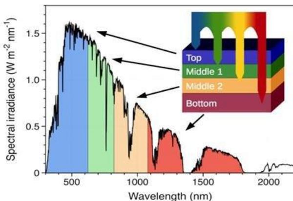
Figure 5: Multi Junction Solar Cell (Singh and John, 1997) The next approach for high performance solar cell and most
