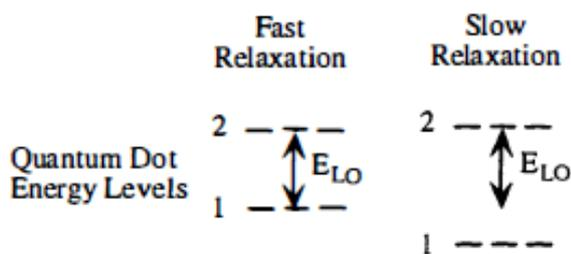
Figure 13: Optical phonon scattering process in bulk and the quantum dot
