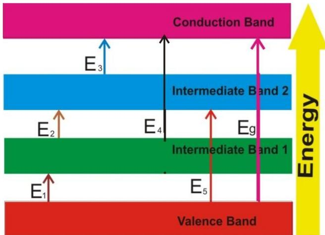
Figure 23: Two Intermediate Band Solar Cell Mechanism with the possible Electronic Transitions.
