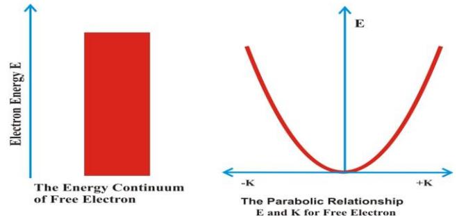
Figure 16: (a) Energy Continuum for Free Electron and (b) Dispersion Relation
