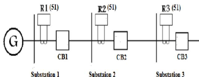
Fig.3 - Radial line supplying three substations.
