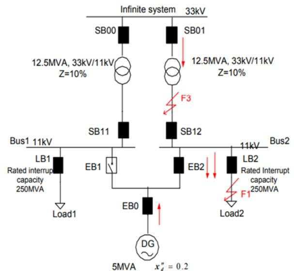
Fig.7 – An alternative network splitting method
