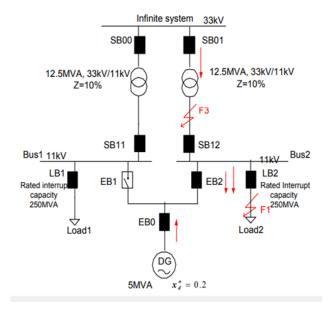
Fig.7 – An alternative network splitting method
