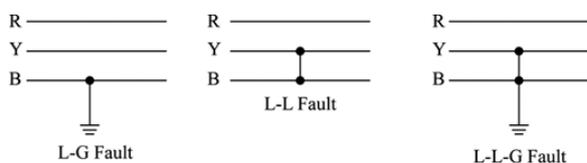
Fig 2 :- Unsymmetrical fault
