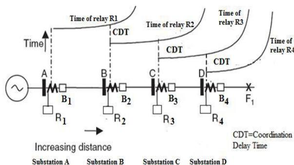
Fig 4:- relay coordination principle.
