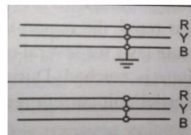
Fig 1 :- Symmetrical fault
