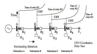
Fig 4:- relay coordination principle.
