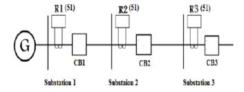
Fig.3 - Radial line supplying three substations.
