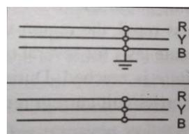
Fig 1 :- Symmetrical fault
