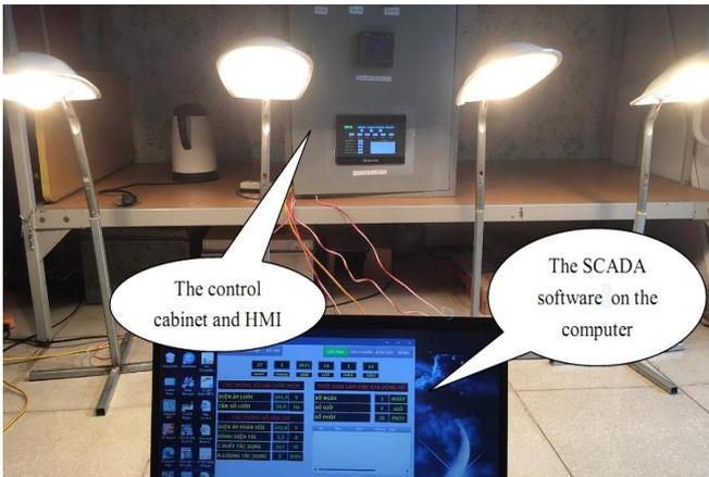
Fig7. The SCADA software of the street lighting energy-saving system
