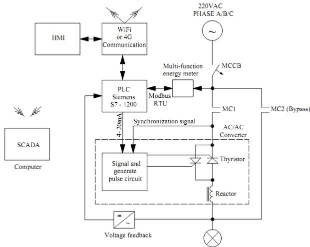
Fig1. Diagram of single-phase control structure
