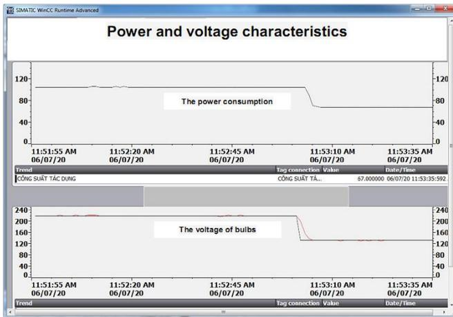
Fig9. 40 percent of the power is reduced at the off-peak time in the standard mode and all bulbs are still on
