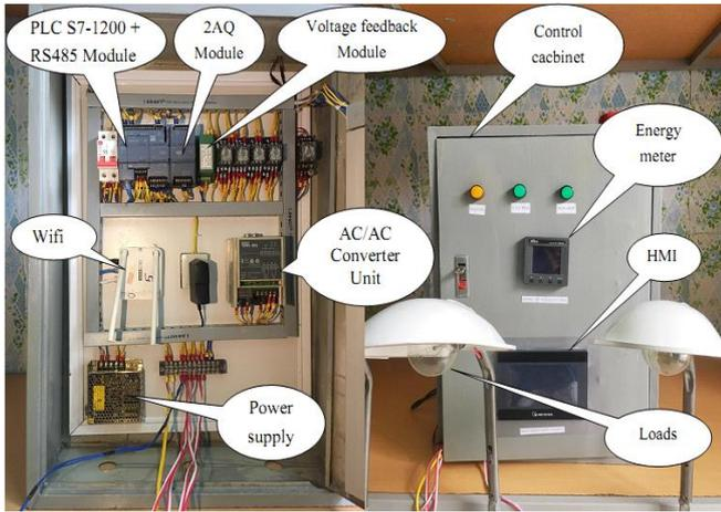
Fig6. The experimental model of the street lighting energy-saving system
