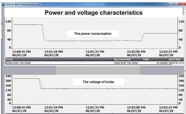
Fig 11. Power characteristics in the mixed mode
