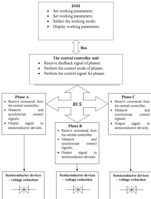
Fig2. The detailed functional diagram of each unit in the street lighting energy-saving system
