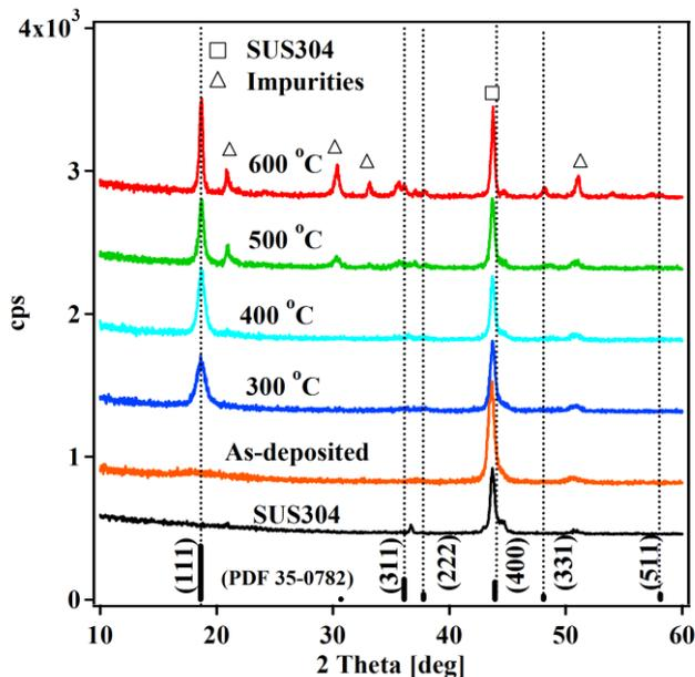
**Figure 1** XRD patterns of  $\text{LiMn}_2\text{O}_4$  thin films annealed at various temperatures.
