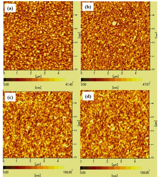
**Figure 3** AFM topographic images of  $\text{LiMn}_2\text{O}_4$  thin films annealed at various temperatures: (a) as-deposited, (b)  $300^\circ\text{C}$ , (c)  $400^\circ\text{C}$  and (d)  $500^\circ\text{C}$ , respectively.
