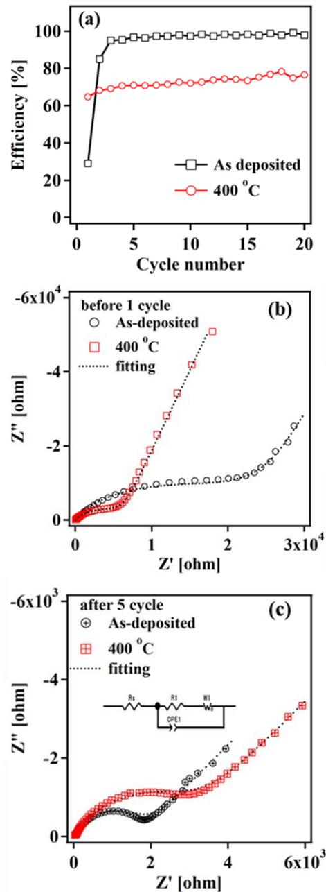
**Figure 6** (a) Coulombic efficiency, (b) and (c) Complex impedance spectra of thin film batteries with the as-deposited cathode film and the cathode film annealed at 400 °C. Inset in Fig. 6c shows circuit elements used for the modeled fitting.
