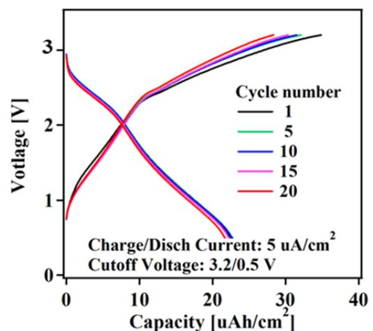
**Figure 4** Charge-discharge curves of a thin film battery with the cathode film annealed at  $400^\circ\text{C}$ .
