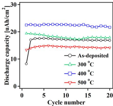
**Figure 5** Cycle performance of thin film batteries with the cathode films annealed at various temperatures.
