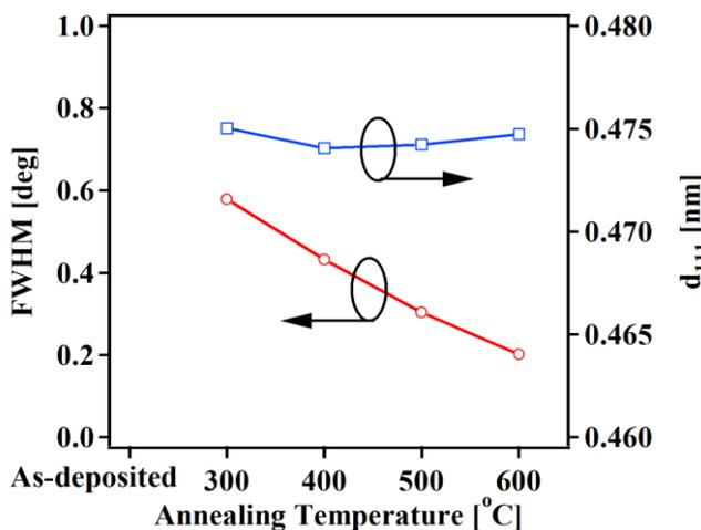
**Figure 2** Dependence of  $d_{111}$  and FWHM of (111) peak of  $\text{LiMn}_2\text{O}_4$  thin films on annealing temperature.
