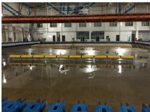
Integral experiment of floating breakwater with flexible structure
