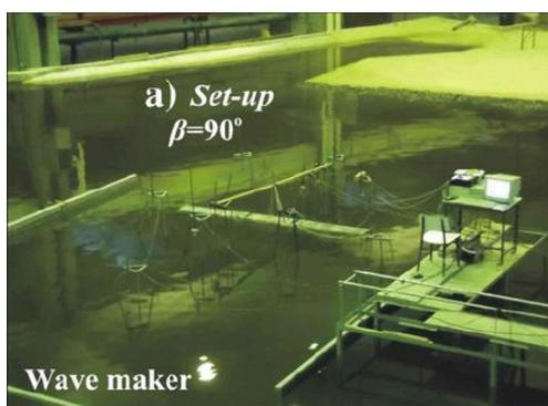
Fig. Experiment on integrated system of pontoon breakwater under transverse and oblique waves
