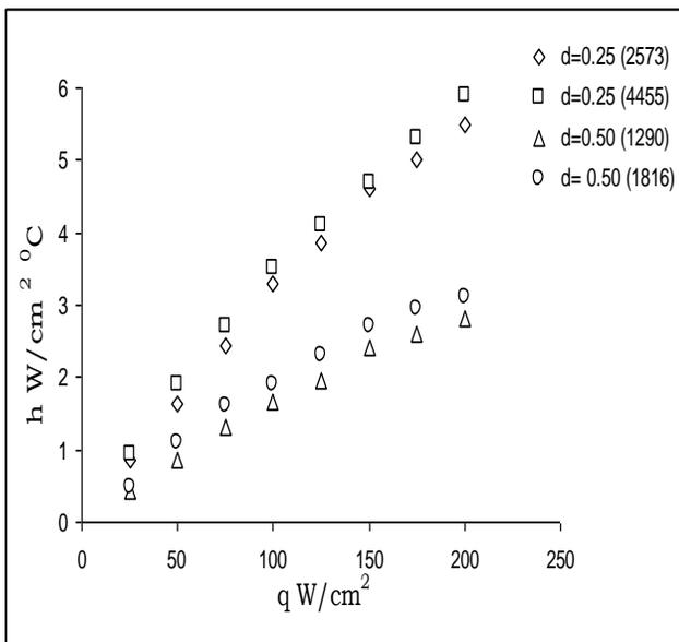
Fig. 2 Variation of heat transfer co-efficient with heat flux for different Reynolds numbers for a horizontal jet at  $Z=20\text{mm}$
