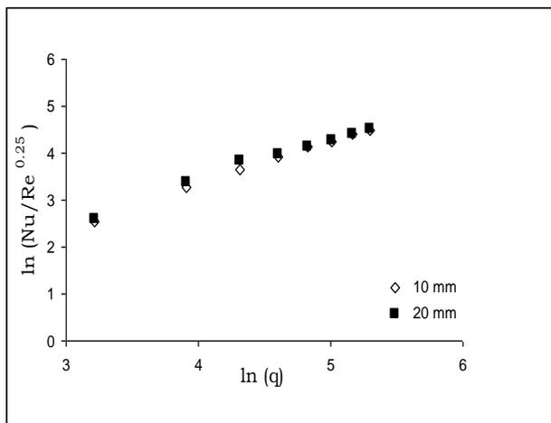
Fig.6 Variation of  $(Nu/Re^{0.25})$  with heat flux at  $Re=1816$ ,  $d=0.50mm$  and  $Z=10$  and  $20mm$  for vertical jets.
