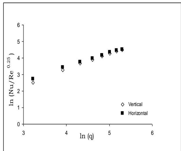
Fig.5 Variation of  $(Nu/Re^{0.25})$  with heat flux at  $Re=1570$ ,  $d=0.50\text{mm}$  and  $Z=20\text{mm}$  for both vertical and horizontal jets
