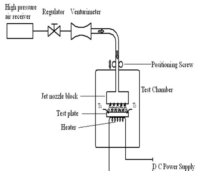
Fig.1(a) Schematic diagram of the experimental set up
