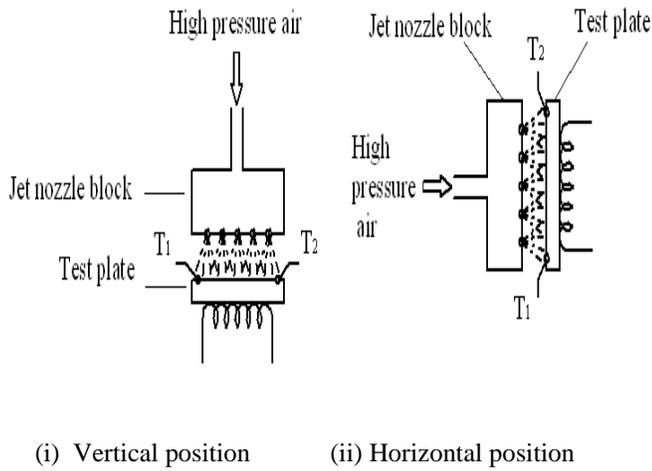
Fig.1(b) Two different positioning of jet nozzle
