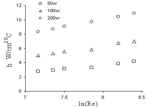
Fig 3 Variation of heat transfer co-efficient with Reynolds numbers at various values of heat flux
