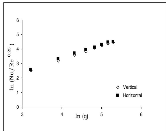
Fig 4 Variation of  $(Nu/Re^{0.25})$  with heat flux at  $Re=1570$ ,  $d=0.50\text{mm}$  and  $Z=10\text{mm}$  for both vertical and horizontal jets
