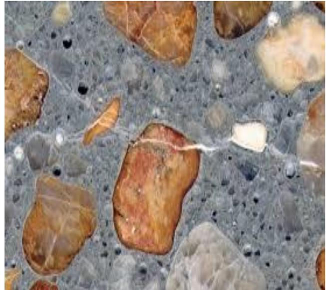
Figure 1. Alkali-silica gel extruded into cracks within the concrete
