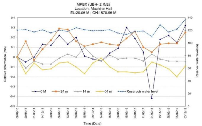
Fig 7: Plot of Relative Deformation Vs Time for MPBX Location UBH-2
