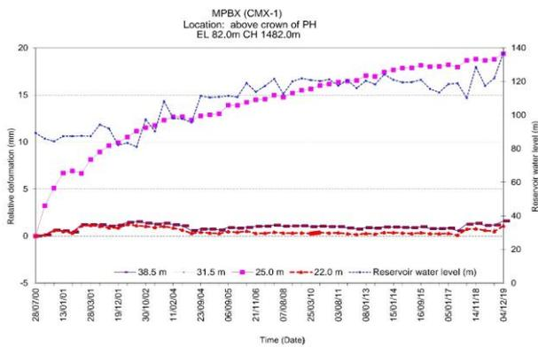
**Fig 9: Plot of Relative Deformation Vs Time for MPBX Location CMX-1**
