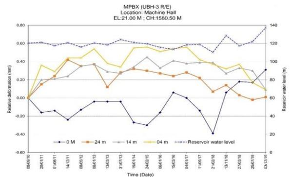
Fig 8: Plot of Relative Deformation Vs Time for MPBX Location UBH-3
