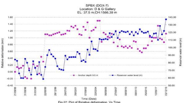
**Fig 12: Plot of Relative Deformation Vs Time for SPBX Location DGX-7**
