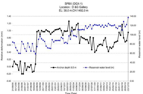
**Fig 11: Plot of Relative Deformation Vs Time for SPBX Location DGX-1**
