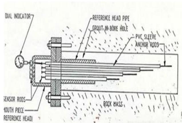
Fig. 2: Typical Multi position borehole extensometer (MPBX)
