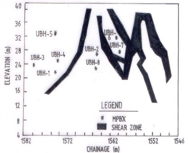
Fig. 5: Instrumentation on upstream wall of powerhouse cavern along with shear
