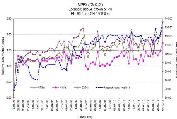
**Fig 10: Plot of Relative Deformation Vs Time for MPBX Location CMX-2**
