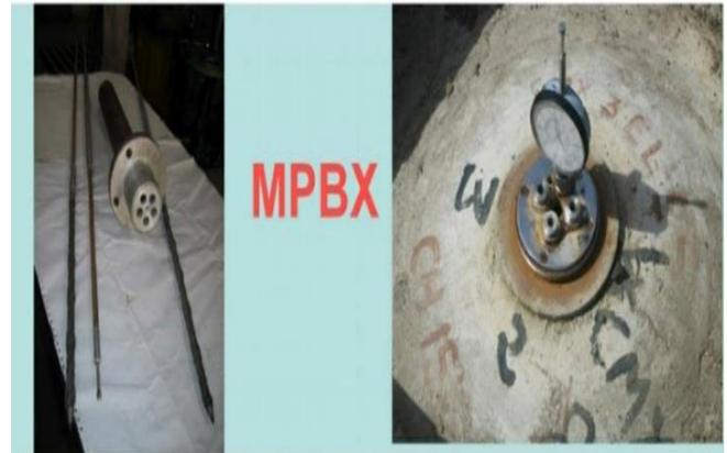
Fig. 1: Multi point borehole extensometer (MPBX) fabricated in CSMRS
