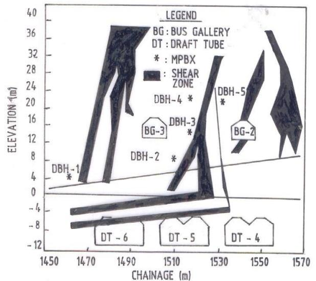
Fig. 6: Instrumentation on upstream wall of powerhouse cavern along with shear zone
