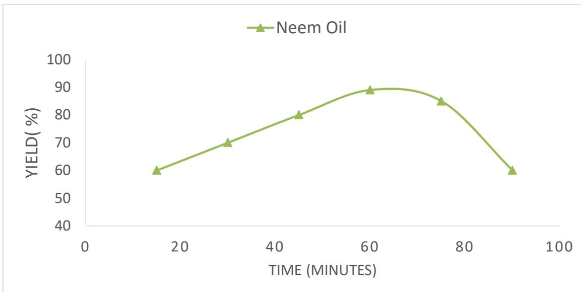
Figure 6: Effect of reaction time on biodiesel yield
