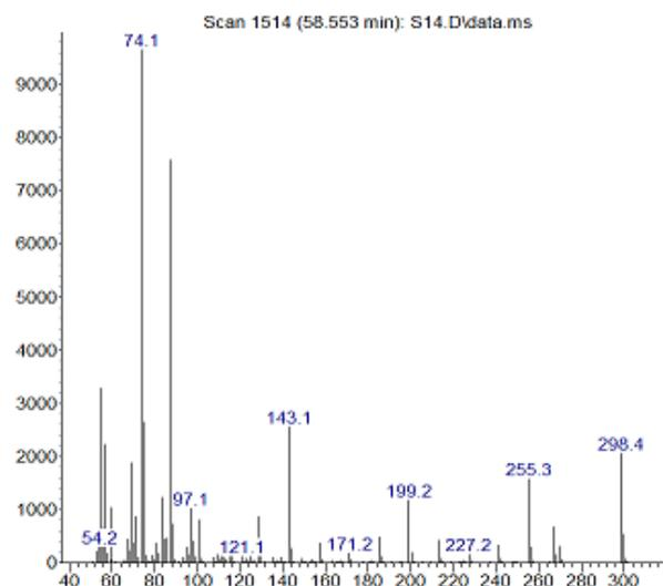
Figure I: GC-MS spectra of neem seed oil.
