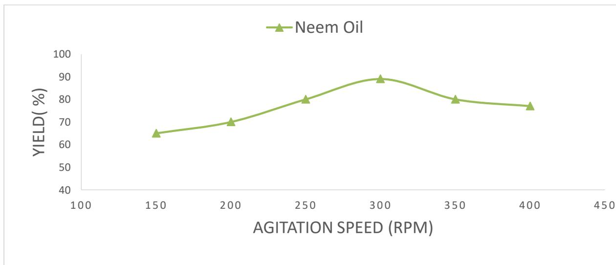
Figure 7: Effect of agitation speed on biodiesel yield.
