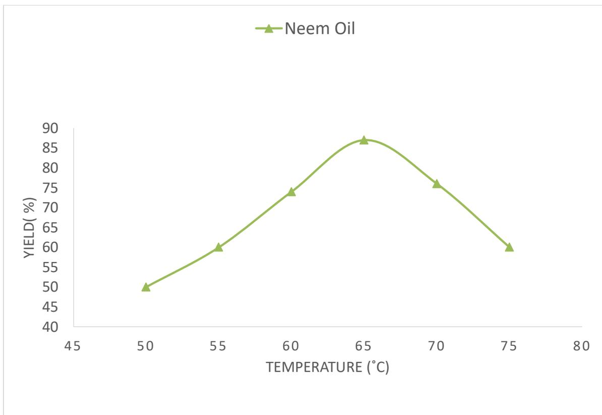
Figure5: Effect of temperature on biodiesel yield.
