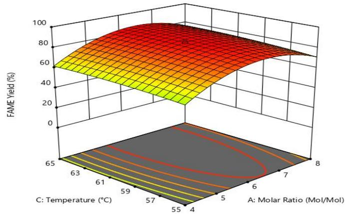
Figure 10: 3D response surface plot showing the effect of methanol/oil molar ratio and temperature on the yield of FAME from neem oil.
