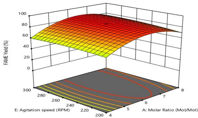
Figure 11: 3D response surface plot showing the effect of methanol/oil molar ratio and agitation speed on the yield of FAME from neem oil.
