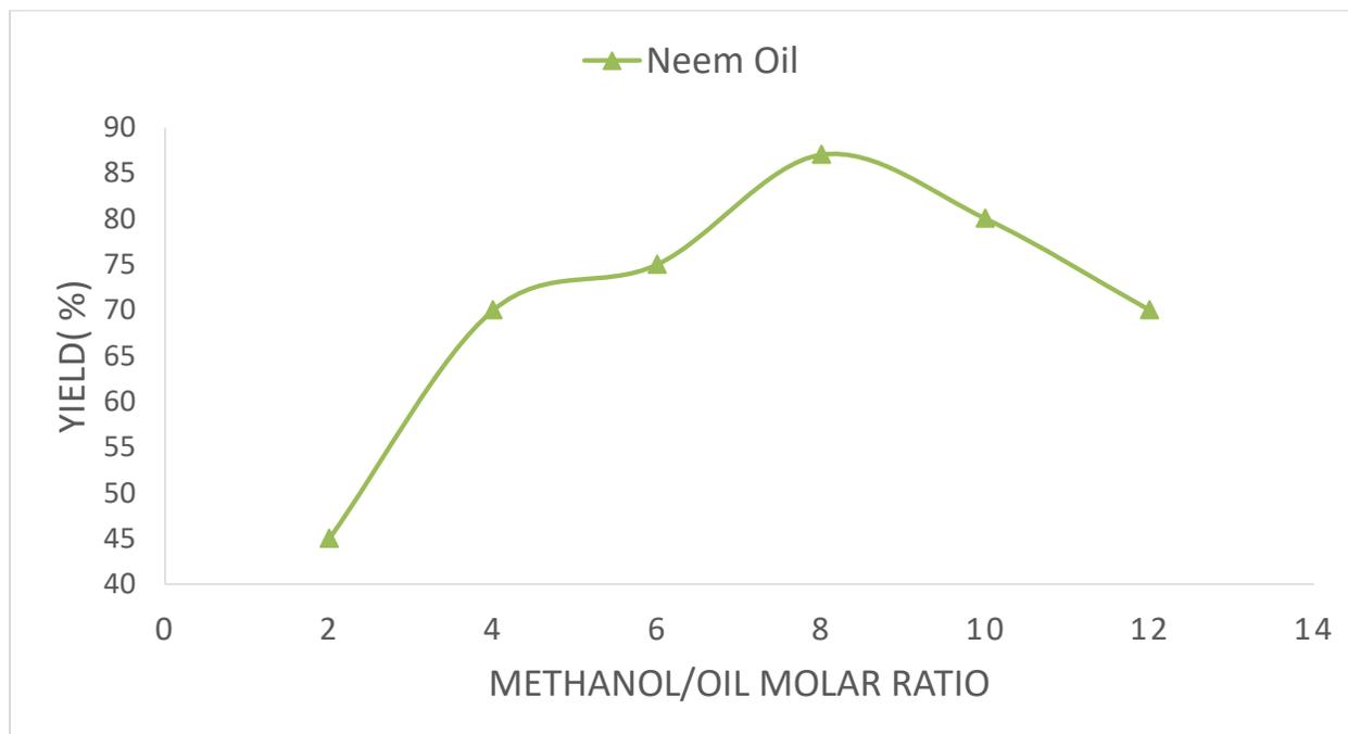
Figure3: Effect of methanol to oil molar ratio on biodiesel Yield.
