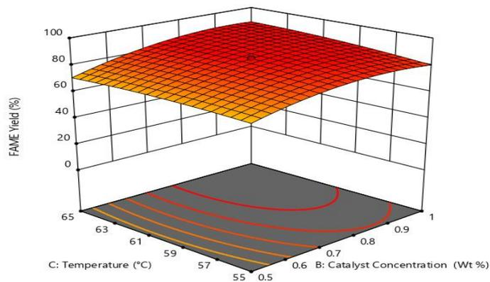
Figure 12: 3D response surface plot showing the effect of temperature and catalyst concentration on the yield of FAME from neem oil.
