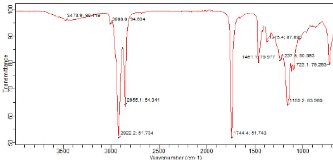
Figure 4.1: FT-IR spectra for neem oil.
