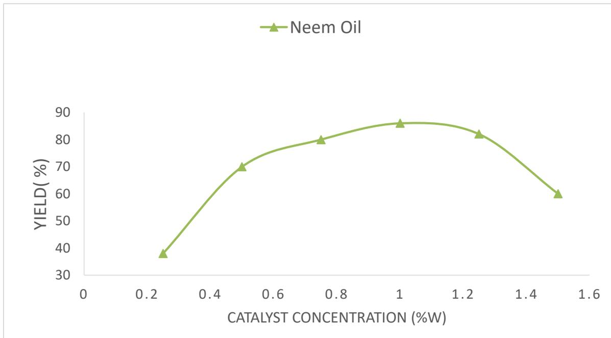
Figure 4: Effect of catalyst concentration on biodiesel yield
