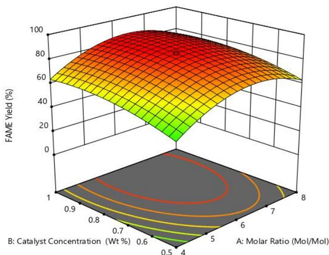
Figure 9: 3D response surface plot showing the effect of methanol/oil molar ratio and catalyst concentration on the yield of FAME from neem oil.
