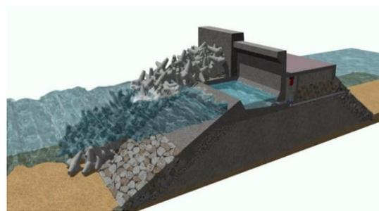
(a) Bottom mounted breakwater
