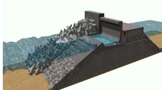
(a) Bottom mounted breakwater
