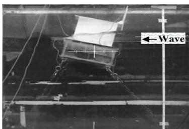
(b) Inclined anchorage method (60 °)
