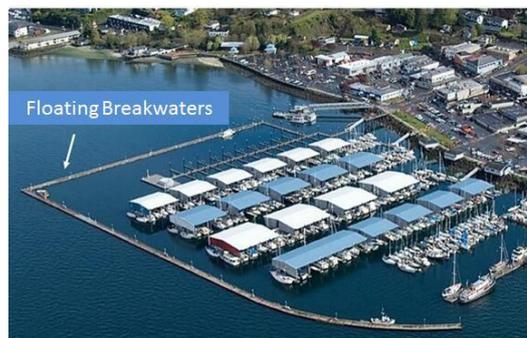
Figure 7 Orchard Harbor Floating Breakwater
