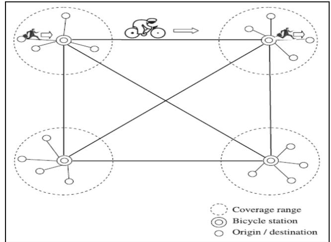
Figure 11 Hub and spoke model of PBSS
