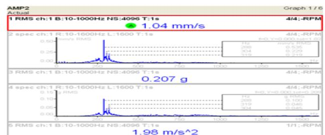
Fig.7: Helical gear with tooth breakage defect with 15 N load at 925 rpm
