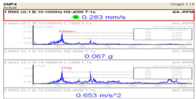
Fig.5: Helical gear with scoring defect with 15 N loads at 925 rpm
