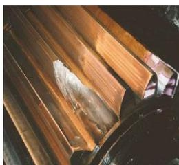
Fig.1: Tooth Breakage Defect
