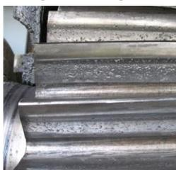
Fig.2: Pitting Defect
