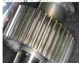
This defect occurs due to lack of lubrication. Due to many reasons
