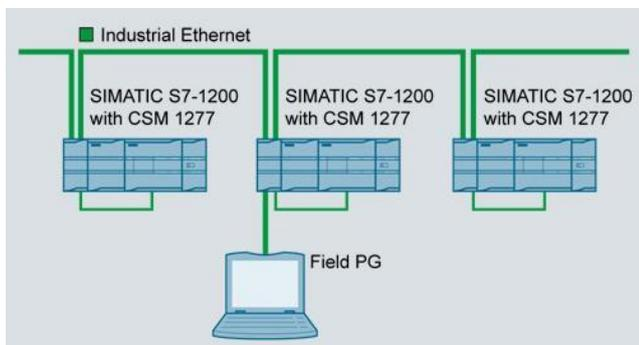
Figure 4. Industrial Ethernet network using PLC S7-1200
