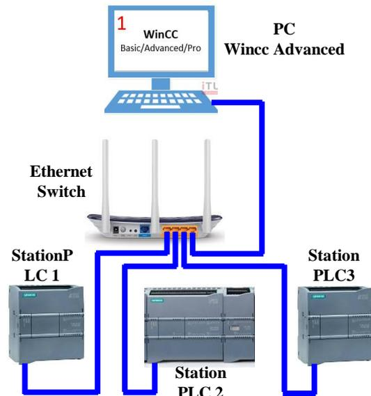
Figure 5. Diagram of control structure
