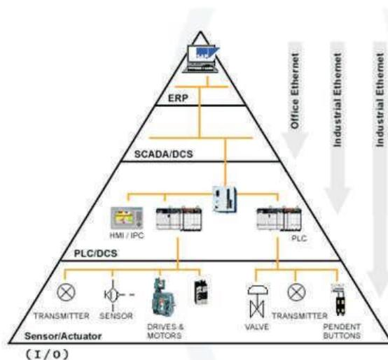
Figure 2. Decentralization of automation systems in industry
