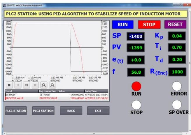
Figure 10. system PLC - Inverter - Motor when changing from 1400 to -1400 rpm
