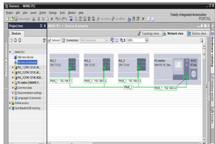
Figure 6. Hardware configuration on TIA Portal software
