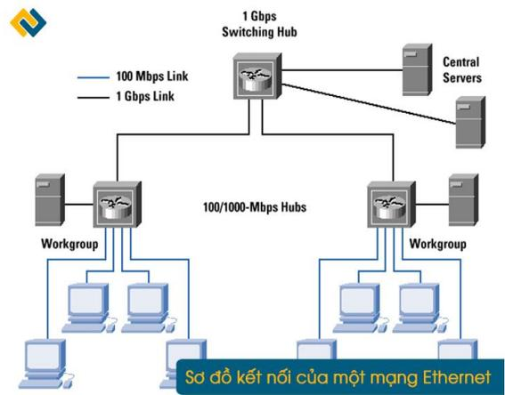
Figure 1. Connection diagram of an Ethernet network
