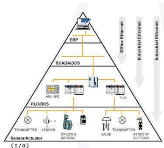
Figure 2. Decentralization of automation systems in industry
