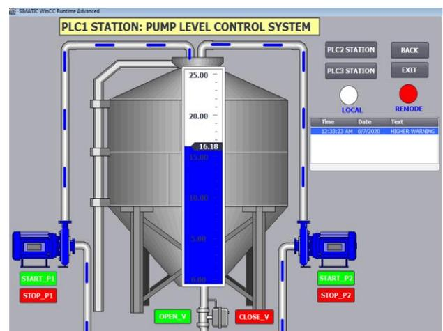
Figure 8. Level control and surveillance
