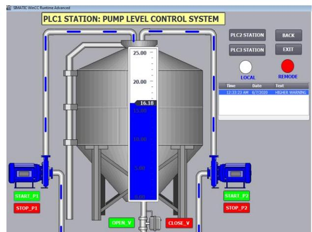
Figure 8. Level control and surveillance
