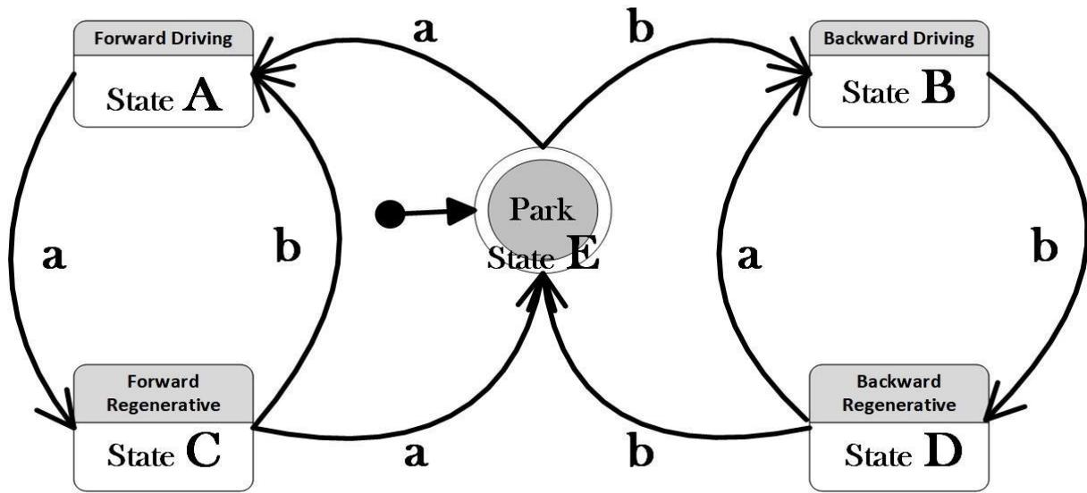
**FIGURE 4. DIAGRAM OF TRANSITION BETWEEN DIFFERENT STATES**
