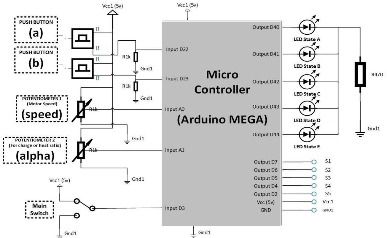
**FIGURE 5A. DETAILED CONTROL CIRCUIT DIAGRAM**
