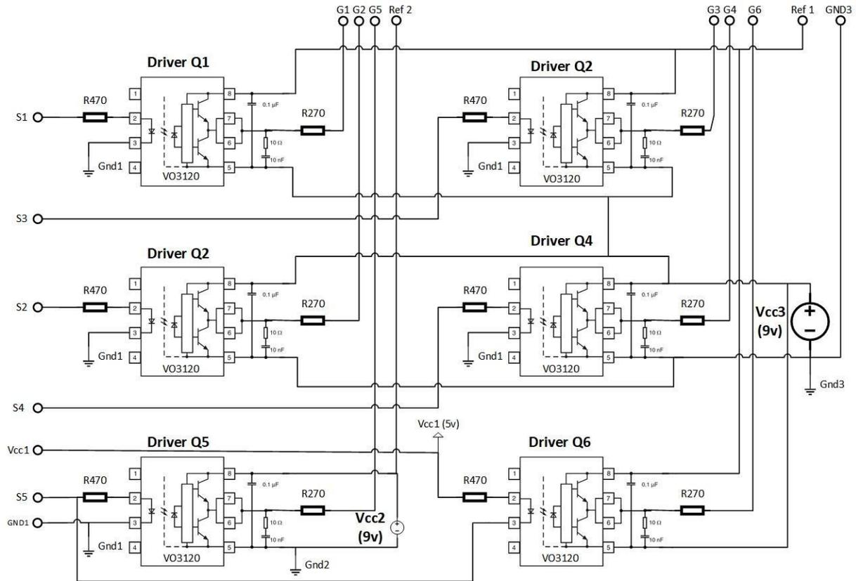
**FIGURE 5B. DETAILED CIRCUIT FOR DRIVING MOSFETS**
