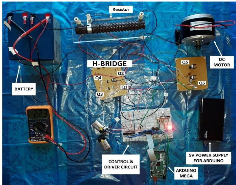
**FIGURE 6 - A VIEW OF THE EXPERIMENTAL SET UP**
