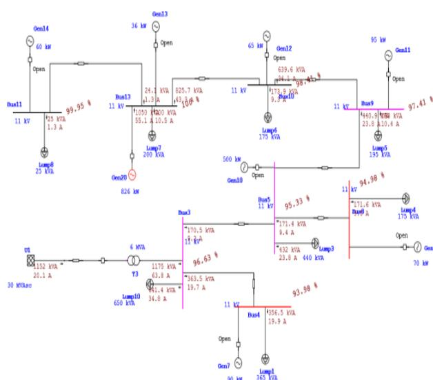
Figure 24: Load flow analysis of power system when DG to Bus 13
