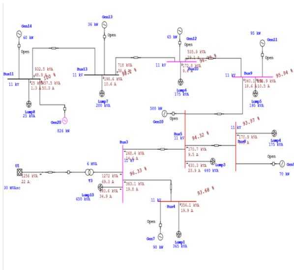
Figure 23: Load flow analysis of power system when DG to Bus 11
