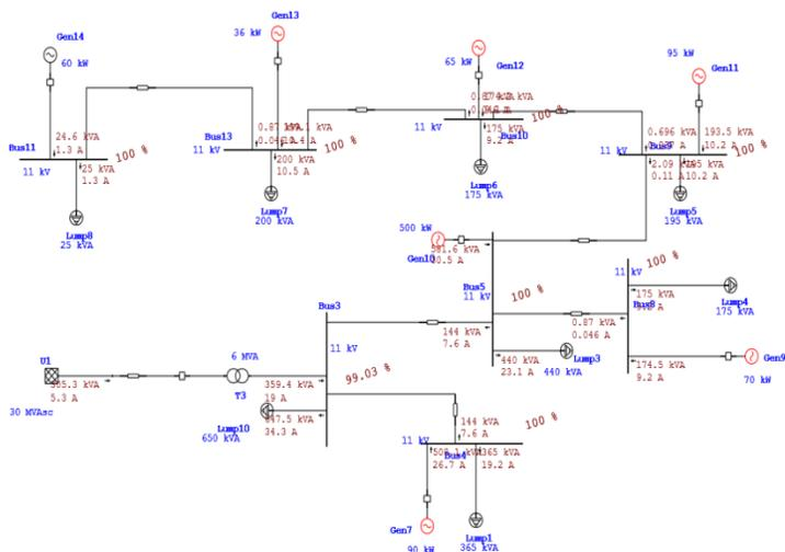
Figure 9: Load flow analysis for LDG, Mini grid and Chimal MHP Plant.
