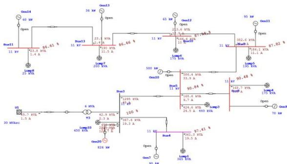
Figure 17: Load flow analysis of power system when DG to Bus 3
