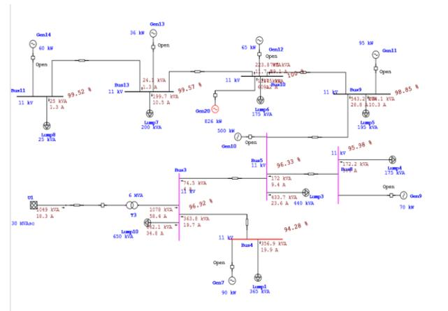
Figure 22: Load flow analysis of power system when DG to Bus 10
