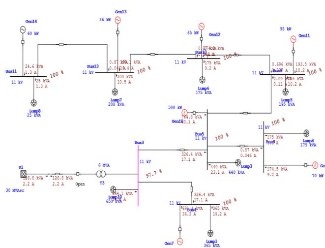
Figure 8: Load flow analysis for Mini-grid and Chimal MHP (90 KW).
