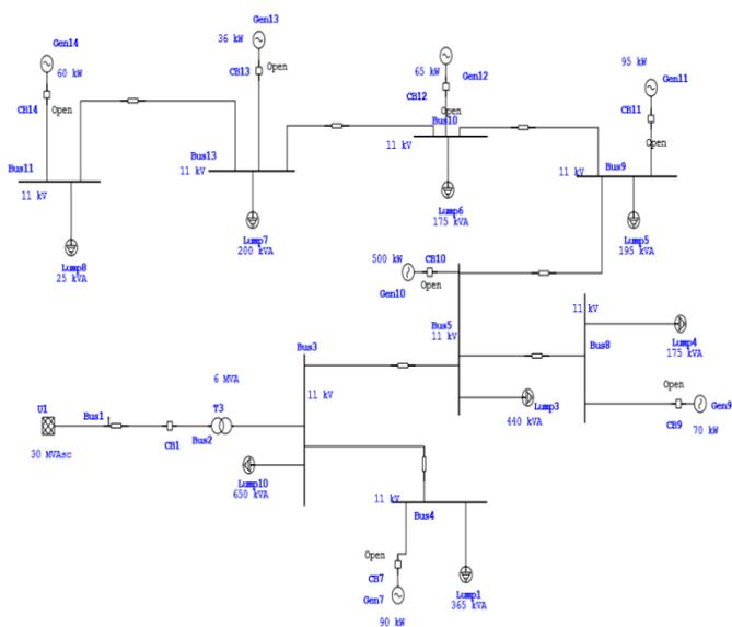
Fig.3 Single Line Diagram of System
