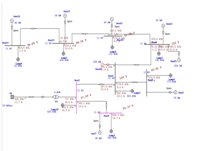
Figure 21: Load flow analysis of power system when DG to Bus 9
