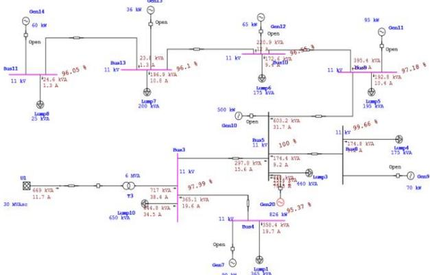
Figure 19: Load flow analysis of power system when DG to Bus 5
