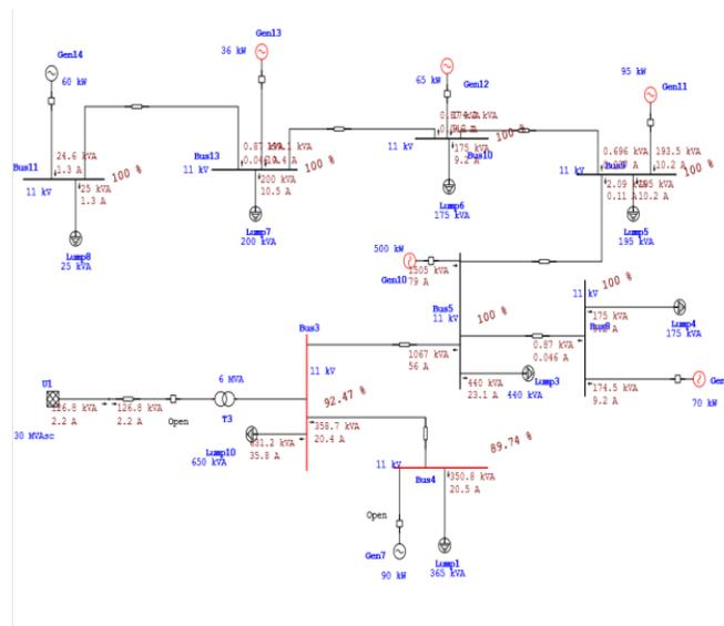
Figure 10: Simulation Diagram for Mini Grid Only.
