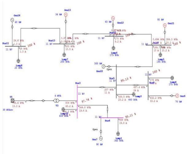
Figure 7: Load flow analysis for Local Distribution Grid (LDG) and Without 500 KW MHP Plant .
