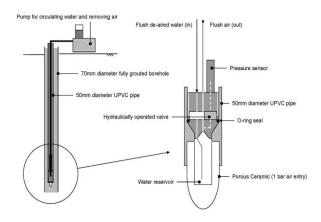
Fig 3-Hydraulic Piezometer
