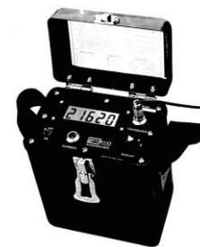
Fig 6- Vibrating Wire Read out unit
