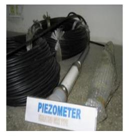
Fig 5-Vibrating Wire Piezometer in CSMRS
