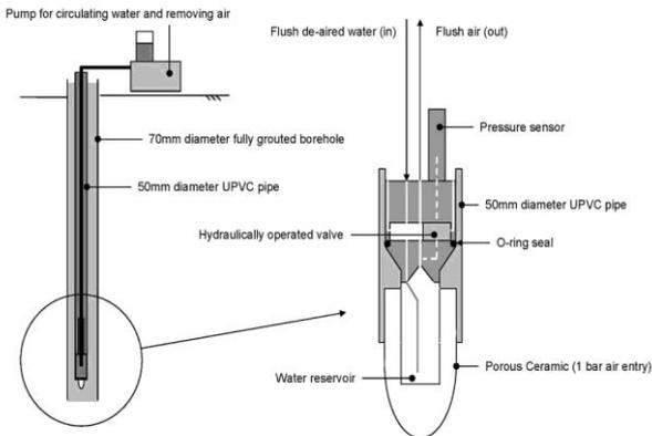
Fig 3-Hydraulic Piezometer
