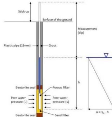
Fig 1-Open Tube Piezometer
