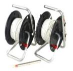
Fig 2-Water Level Indicator/Sounder
