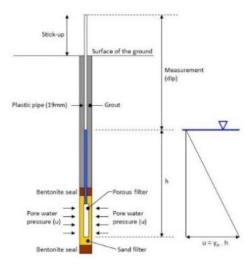
Fig 1-Open Tube Piezometer
