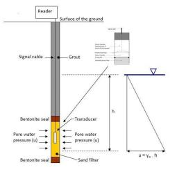
Fig 4-Vibrating Wire Piezometer
