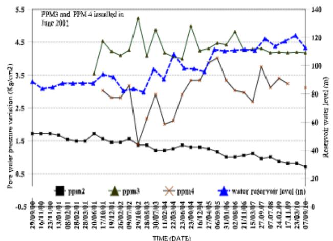
Fig 8<sup>6</sup>: Pore water pressure variation graph in correlation with reservoir water level
