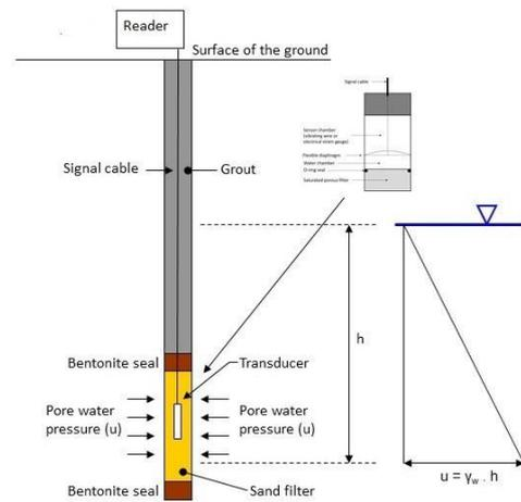
Fig 4-Vibrating Wire Piezometer
