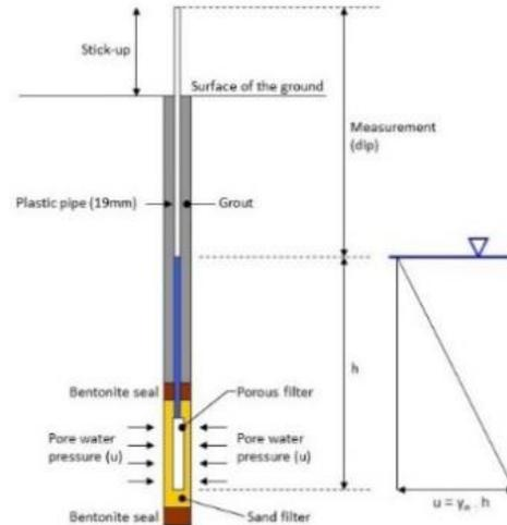
Fig 1-Open Tube Piezometer
