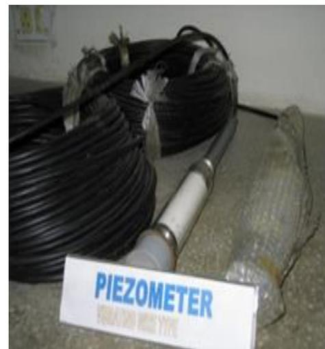
Fig 5-Vibrating Wire Piezometer in CSMRS
