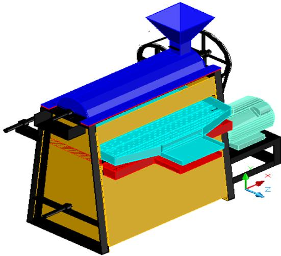
Fig.5. SE Isometric view of rice destining machine
