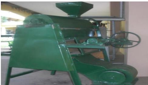
Plate.1. Picture of fabricated rice destining machine
