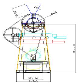
Fig. 2. Orthographic View of Rice destining machine
