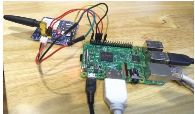
Fig 7. SIM900A Module for mobile phone communication
