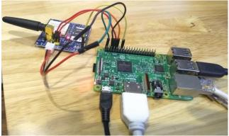
Fig 7. SIM900A Module for mobile phone communication
