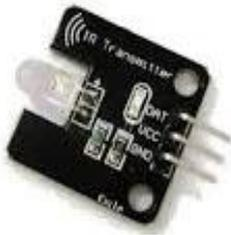
Fig 4. IR-T940 Infrared remote module
