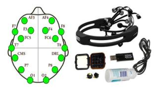
Fig.2. Emotiv Epoc+ headset and 16 electrodes location
