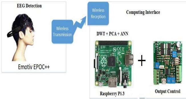
Fig 3. EEG based Controller
