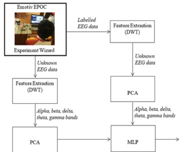
Fig 8. Diagram of functions in control software
