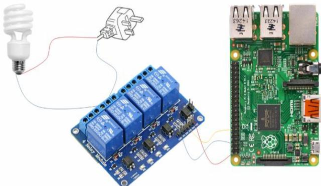
Fig 5. Relay Module for turning on / off the lights
