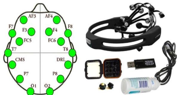
Fig.2. Emotiv Eloc+ headset and 16 electrodes location
