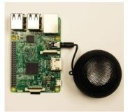
Fig 6. Speaker command module for relative calling
