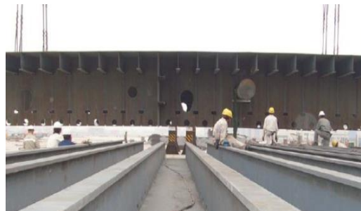
Fig.2 Illustration of double-flat floor pull-in method
