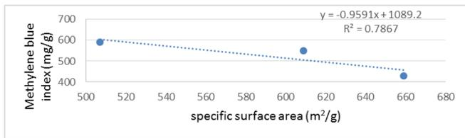
Fig. 8: Correlation between methylene blue index and specific surface area of coals
