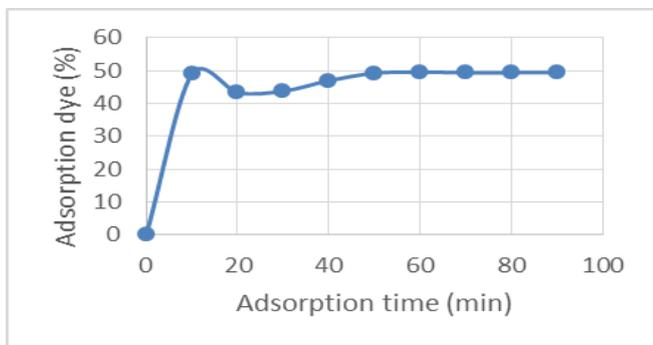
Fig. 10: Kinetics of adsorption of red methyl
