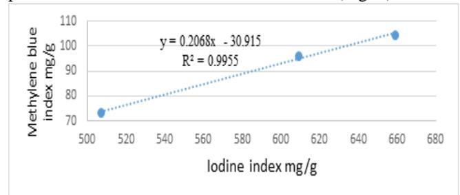
Fig. 5: Correlation between iodine index and methylene blue index of coals
