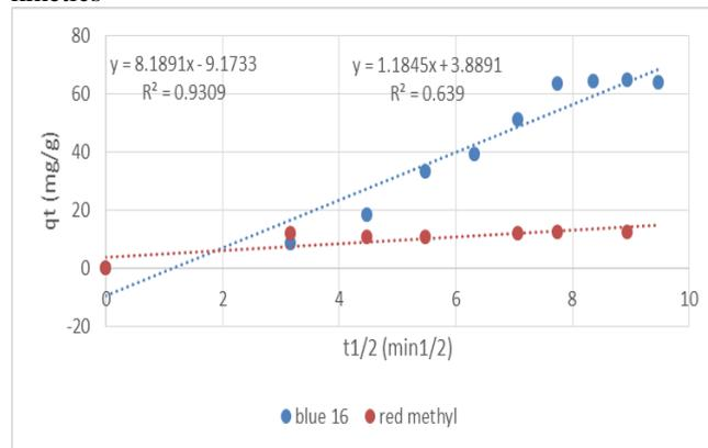
Fig. 13: Model of intraparticle diffusion of adsorption kinetics of dyes
