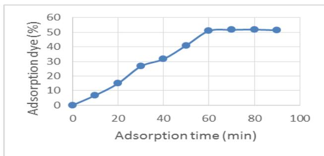
Fig. 9: Kinetics of adsorption of blue 16
