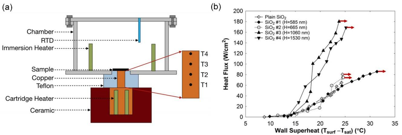
Fig. 3 (a) Experimental setup used for studying pool boiling with porous structure (sample) as heat transfer surface heated using copper rod and water enclosed in chamber [21] (b) Heat flux versus wall super heat showing the higher CHF attained by using micro and nano meters scale structures for heat transfer during phase change at boiling [23]
