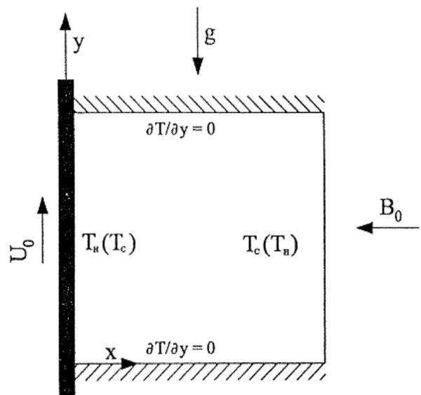
Fig. 2 Schematic of square lid-driven cavity with lid velocity ( $U_0$ ) and magnetic field ( $B_0$ ) to study MHD flow [10].
