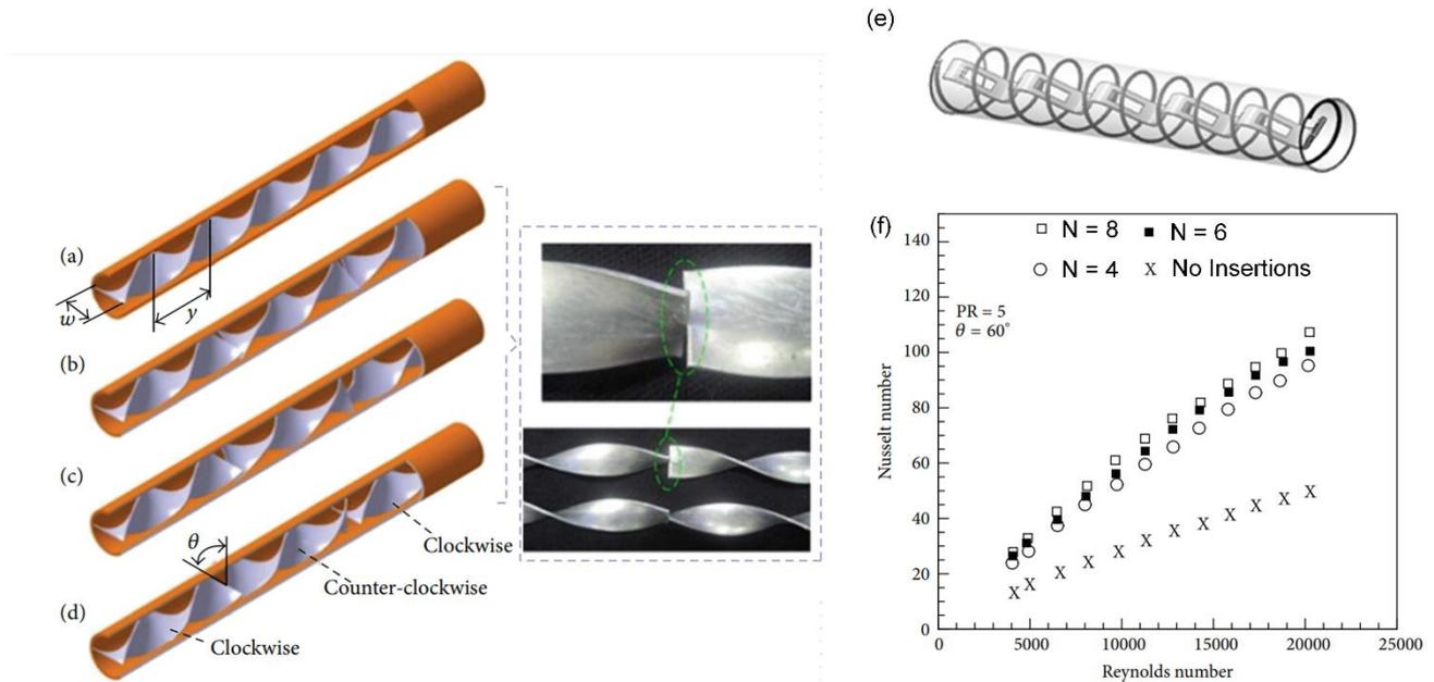
Fig. 1 (a-d) Sketch of clockwise and counter-clockwise twisted tape used as insertions for heat transfer enhancement [7]. (e) Combined wire coil and wavy strip used for insertion [8]. (f) Variation of Nusselt number with Reynolds number for different number of blades  $N$  in insertions used at given pitch ratio  $PR$  and blade angle  $\theta$  [9]
