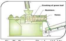
Fig. 2b: Rotorvane Sketches [1], [4]
