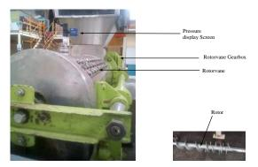
Plate 2: Rotorvane fitted with pressure gauge [1], [4]
