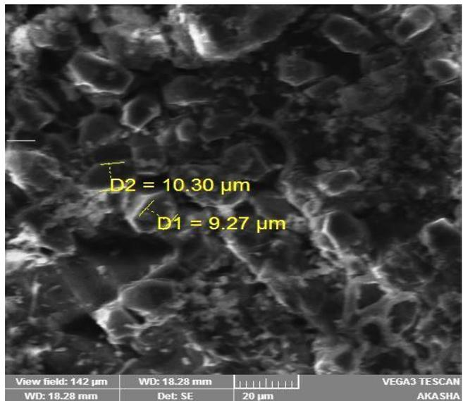
Figures (6). SEM micrograph of mesquite fibers.
