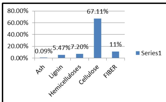
Figure 3. chemical composition of the produced mesquite fiber.
