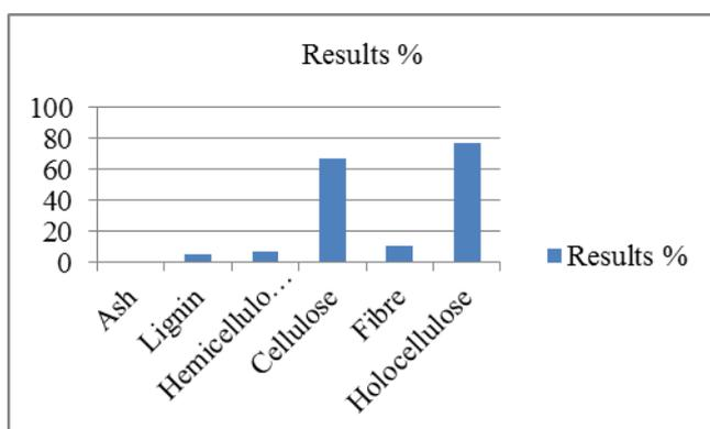
Figure 1 Chemical composition of Raw Material (mesquite stalk).
