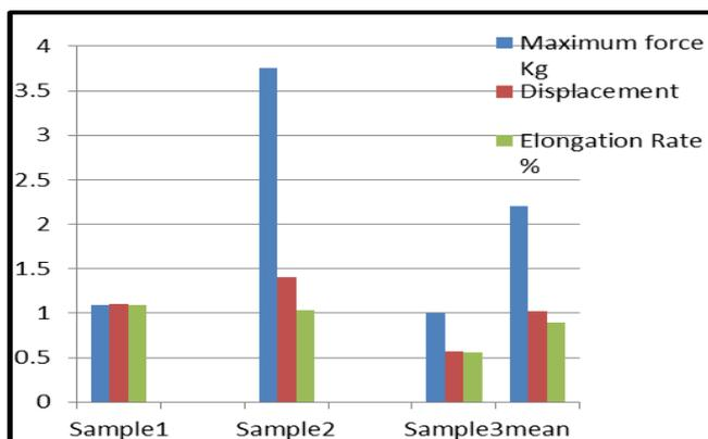
Figure 5. Tensile testing of mesquite fiber samples.
