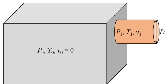
Figure 1. System for the extraction of air from a room.  $P$  is the pressure,  $T$  the temperature,  $v$  the gas velocity and  $D$  is the diameter of the extraction tube
