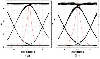
Fig.7. Eye diagrams of DIM code at (a) 50 km (b) 100 km
