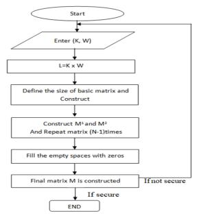
Fig.1. Flow chart of Diagonal identity matrix codes
