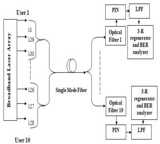
Fig.2. Block diagram of proposed OCDMA system using DIM codes for 10 users at 5Gbps
