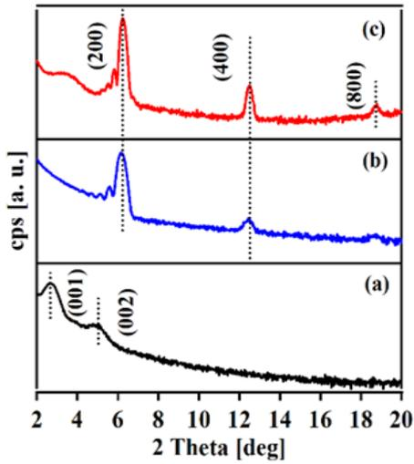
**Figure 2** XRD patterns of (a) DH-α6T thin film of 5 nm, (b) an F<sub>16</sub>CuPc single layer of 20 nm and (c) a 20 nm/5 nm of F<sub>16</sub>CuPc/DH-α6T bilayer deposited on SiO<sub>2</sub>/Si substrates at 120 °C.
