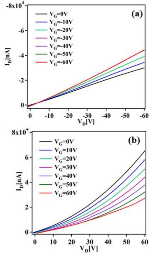
**Figure 4** Output characteristics of F<sub>16</sub>CuPc/DH-α6T TFT working in (a) hole-enhancement and (b) electron-depletion modes.
