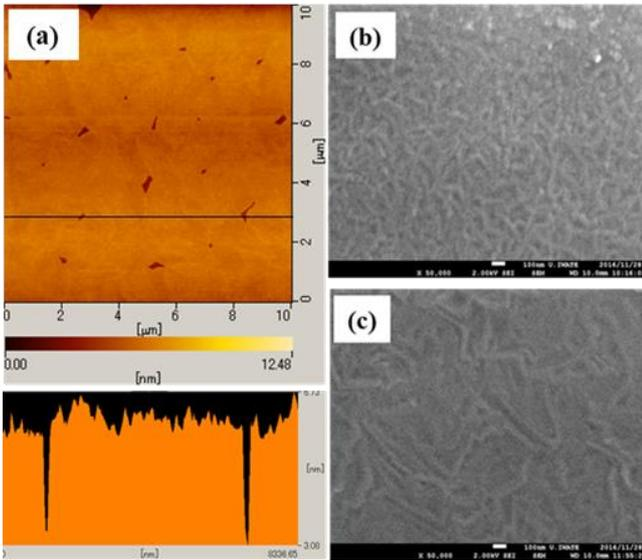
**Figure 3** AFM images of (a) a DH-α6T of 5 nm with cross-sectional profile data corresponding to the black line, the SEM images of (b) the F<sub>16</sub>CuPc single layer of 20 nm deposited on SiO<sub>2</sub>/Si substrate and (c) the 20 nm/5 nm of F<sub>16</sub>Pc/DH-α6T bilyer (All thin films deposited on SiO<sub>2</sub>/Si substrates at 120 °C).
