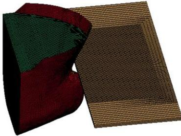
Fig. 1.3 Finite element model of collision between bow and ice row
