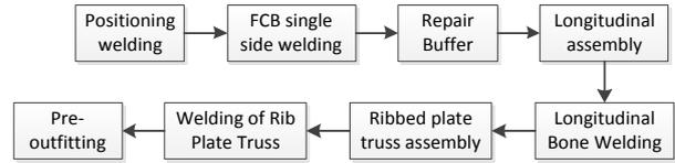
Fig. 3 Schematic diagram of the plane segmentation pipeline
