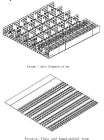
Fig.4 Sectional anatomical diagram of double bottom plane
