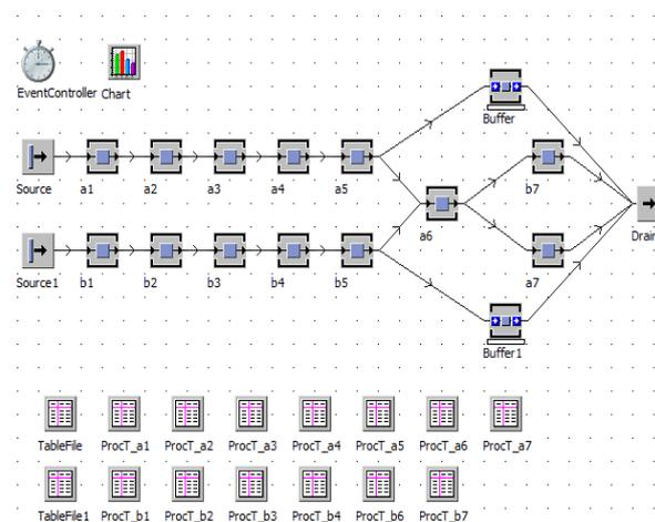
Fig. 7 Optimization Simulation Pipeline Modeling
