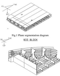
Fig.2 Surface segmentation diagram
