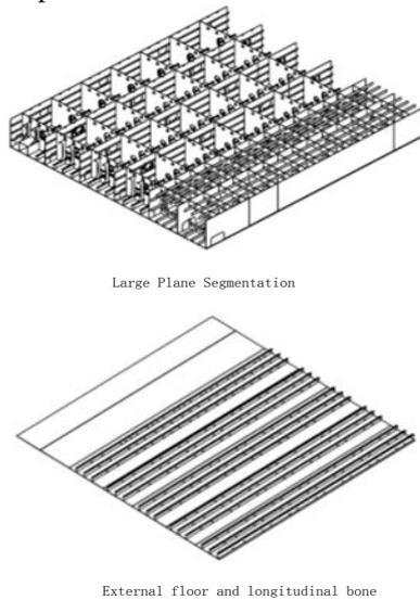
Fig.4 Sectional anatomical diagram of double bottom plane
