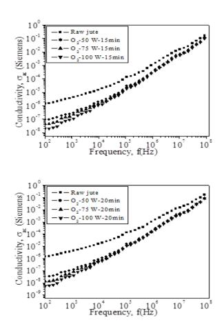
Fig. 4(c) Electrical conductivity,  $\sigma_{ac}$ , as a function of frequency of raw jute and LTP treated jute for various discharge powers at a constant treatment time of O<sub>2</sub> plasma.
