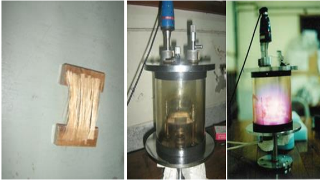
Fig. 1 Schematic diagram of jute fibre and position of it in the glow discharge reactor.
