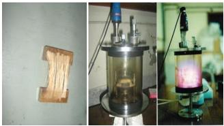
Fig. 1 Schematic diagram of jute fibre and position of it in the glow discharge reactor.
