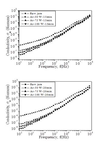
Fig. 4(b) Electrical conductivity,  $\sigma_{ac}$ , as a function of frequency for raw jute and LTP treated jute for various discharge powers at a constant treatment time of Ar plasma.
