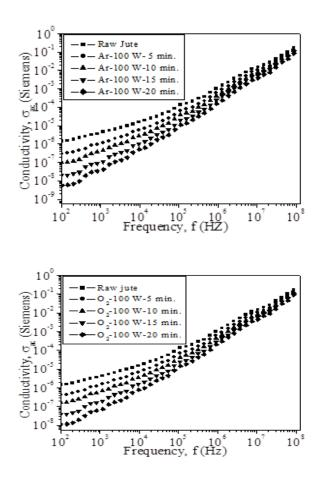
Fig. 4(a) Electrical conductivity,  $\sigma_{ac}$ , as a function of frequency of raw jute and LTP treated jute for various treatment times and discharge powers of Ar and O<sub>2</sub> plasmas.
