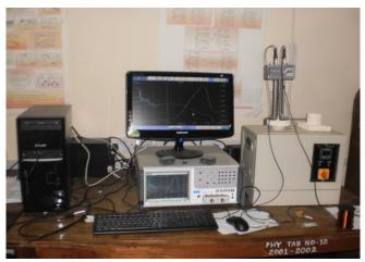
Fig. 3 Arrangement for AC measurement
