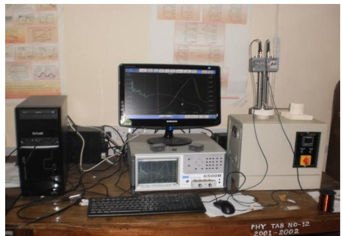
Fig. 3 Arrangement for AC measurement
