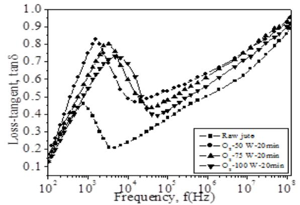
Fig. 4(c): Variation of dielectric loss-tangent with frequency of raw and LTP treated jute at various discharge powers at a constant treatment time for O<sub>2</sub> plasma.
