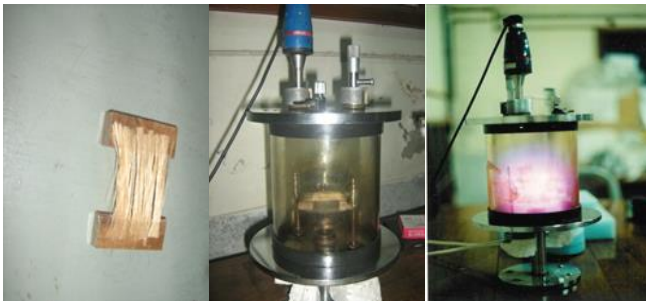
Fig. 1 Schematic diagram of jute fibre and position of it in the glow discharge reactor
