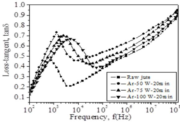
Fig. 4(b): Variation of dielectric loss-tangent with frequency of raw and LTP treated jute at various discharge powers at a constant treatment time for Ar plasma.
