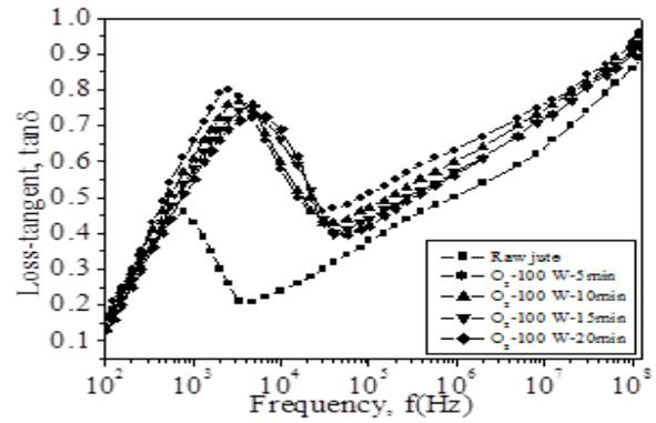
Fig. 4(a): Variation of loss-tangent with frequency of raw and LTP treated jute of various treatment times and discharge powers for Ar and O<sub>2</sub> plasmas.
