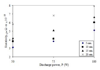
Fig. 6 Resistivity vs. discharge power for Ar plasma at various exposure times
