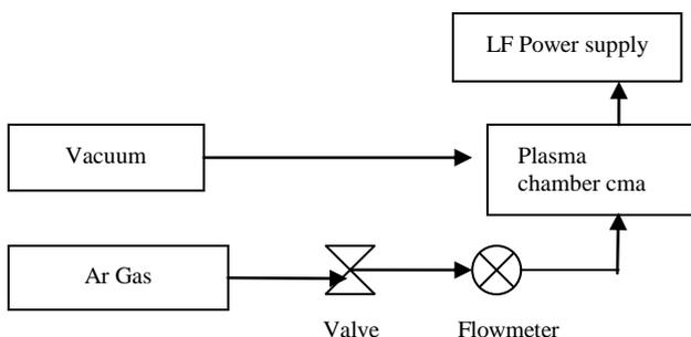
Fig. 2 Flow chart of the plasma treatment set-up
