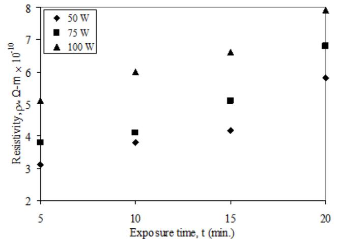
Fig. 7 Resistivity vs. exposure time for Ar plasma at various discharge powers
