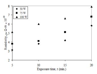
Fig. 7 Resistivity vs. exposure time for Ar plasma at various discharge powers
