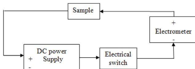
Fig. 3 A schematic block diagrams for room temperature DC measurements
