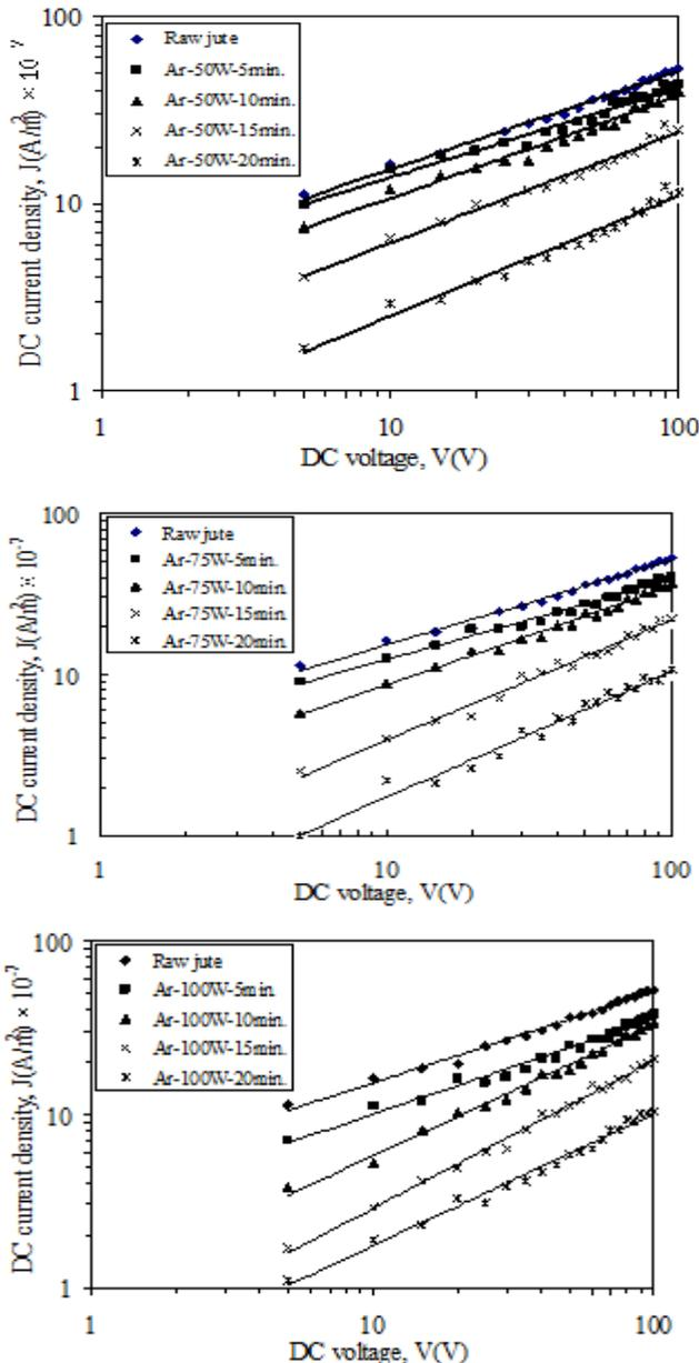
Fig. 5 J-V plots for raw jute and LTP treated jute for Ar plasma at various discharge powers and exposure times.
