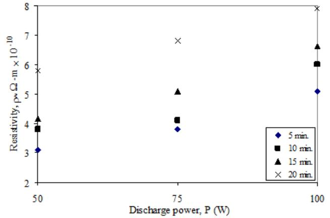
Fig. 6 Resistivity vs. discharge power for Ar plasma at various exposure times
