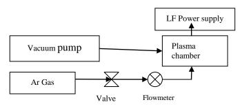
Fig. 2 Flow chart of the plasma treatment set-up
