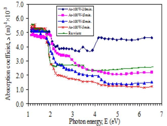
Fig. 5 Absorption coefficient vs. photon energy curves for Ar plasma at different powers and treatment times.
