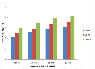
Fig. 6(b) Band gap vs. treatment time of jute in Ar plasma at different discharge powers
