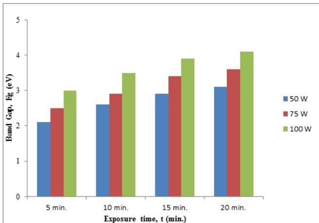
Fig. 6(b) Band gap vs. treatment time of jute in Ar plasma at different discharge powers
