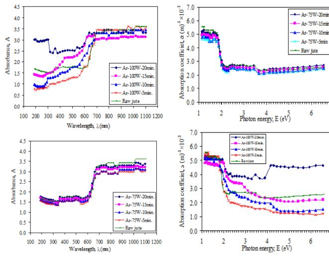
Fig. 4 Absorbance vs. wavelength curves for Ar plasma at different powers and treatment times
