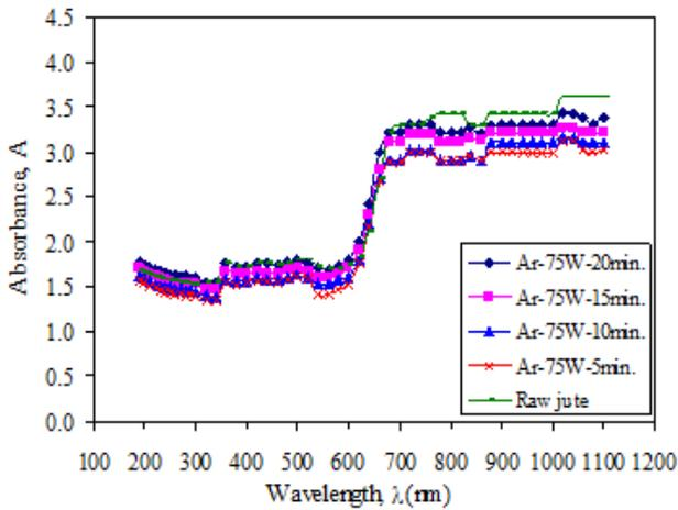
Fig. 4 Absorbance vs. wavelength curves for Ar plasma at different powers and treatment times
