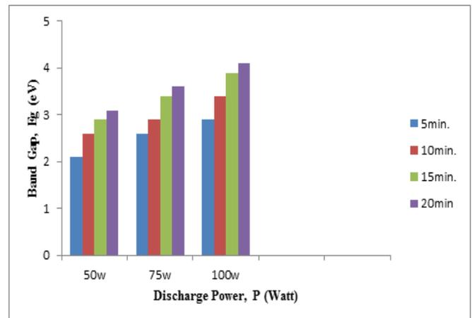
Fig. 6(a) Band gap vs. discharge power of jute in Ar plasma at different times
