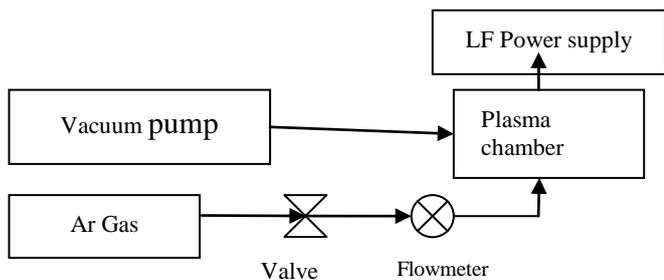
Fig. 2 Flow chart of the plasma treatment set-up
