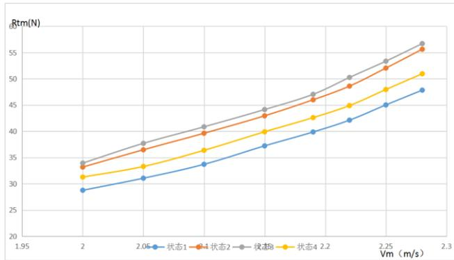
Figure 6 Ship model resistance curve
