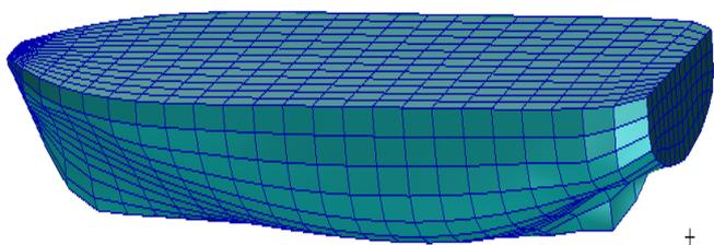
Figure 3 hull model grid specific division
