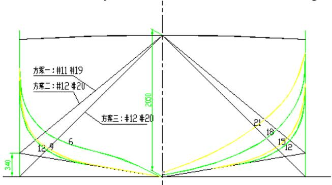
Figure 8 keel installation location
