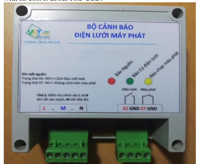
Fig. 10: Actual image of the warning device for running generator (in case the generator is located far away from the BTS)
